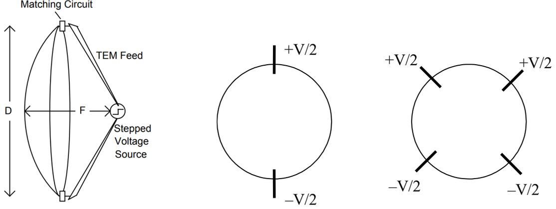
Figure 1. Sketch of a 2-arm IRA (left and center) and a 4-arm IRA (right).
