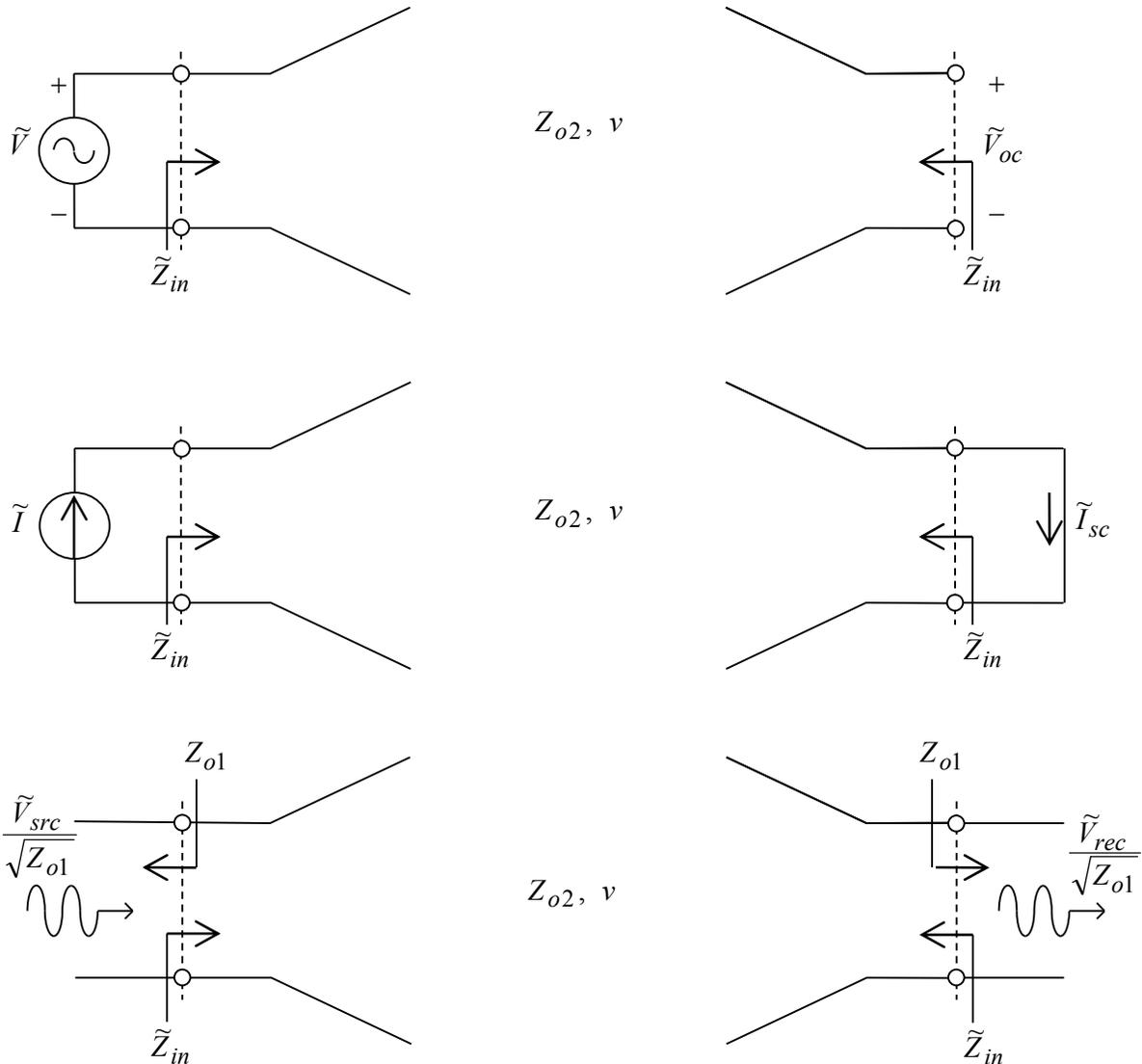
Figure 2.1. Three cases of antenna transmission (left) and reception (right) under conditions of open circuit (top), short circuit (middle), and power wave (bottom).
