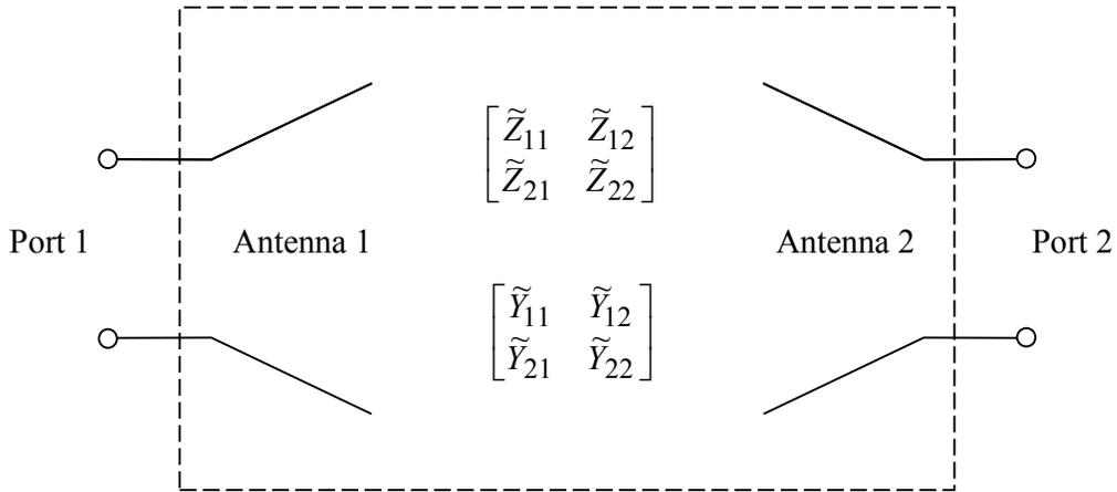
Figure 2.3. Two-port equivalent circuit of a two-antenna system.
