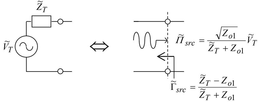
Figure 7.2. The relationship between a Thévenin equivalent source (left) and a power wave source (right) at a port with reference impedance  $Z_{o1}$ .
