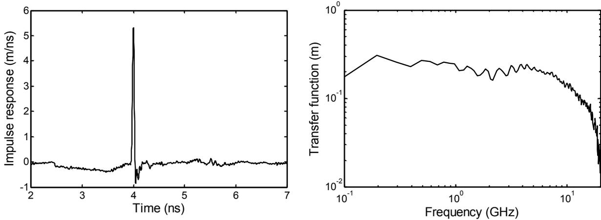
Figure 9.1. Impulse response (left) and transfer function (right) of the IRA-3Q.
