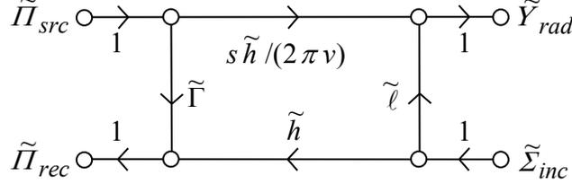
Figure 6.2 Signal flow graph representation of the GASM.
