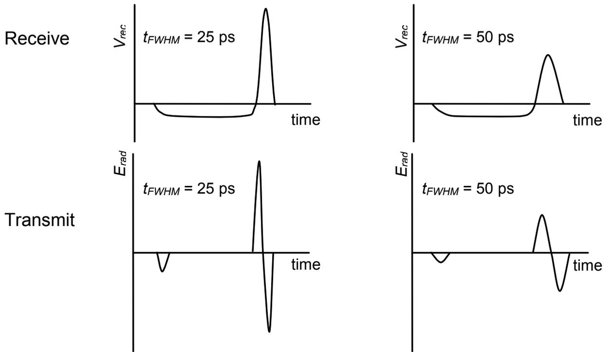
Figure 1.2. Characterizing an Impulse Radiating Antenna on boresight for dominant polarization by its response to an incident infinite plane-wave electric field with Gaussian time dependence (top), and a Gaussian 50- $\Omega$  source voltage (bottom), at two different Gaussian pulse widths (left and right). Note that  $t_{FWHM}$  is the Full-Width Half Max of the incident field or voltage. (Scale is approximate.)
