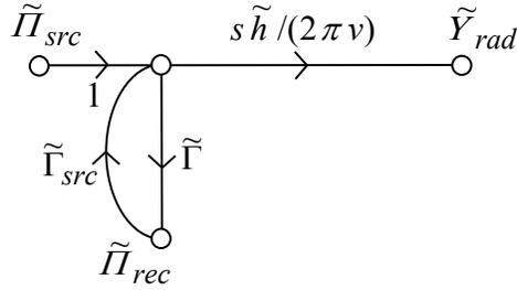
Figure 7.1 Signal flow graph for a source with arbitrary impedance.
