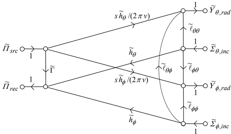
Figure 6.4 Scalar signal flow graph representation of the GASM including both polarizations.
