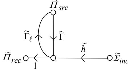
Figure 7.3 Signal flow graph for reception into an arbitrary load.
