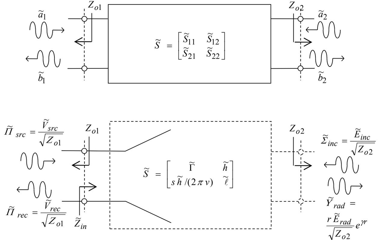
Figure 6.1. The Generalized Antenna Scattering Matrix (GASM), on boresight, for dominant polarization.
