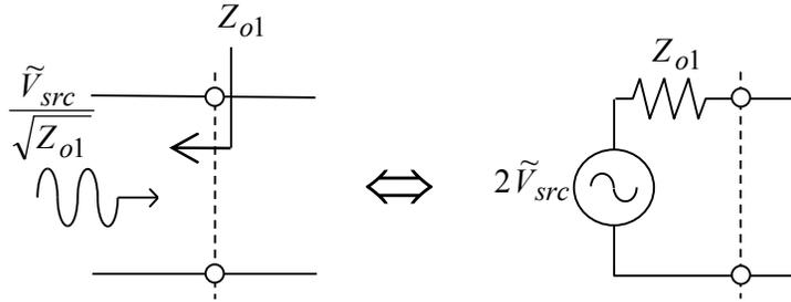
Figure 2.2. Thévenin equivalent circuit of the power wave source voltage.
