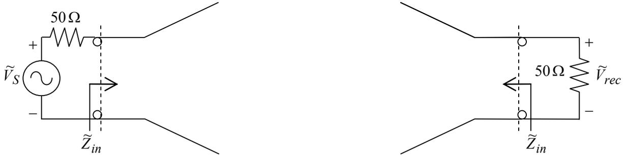
Figure 2.1. Antenna transmission (left) and reception (right) for a  $50\text{-}\Omega$  source and load. Note that  $\tilde{V}_S = 2\tilde{V}_{src}$  in a  $50\text{-}\Omega$  source.
