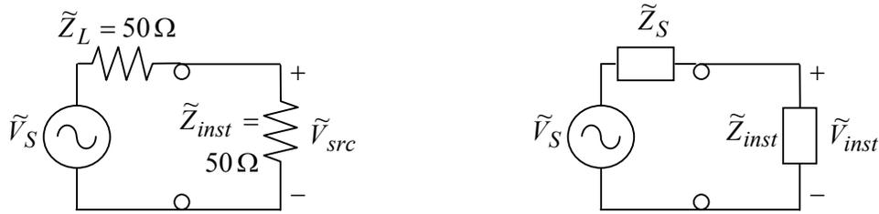
Figure 2.3. Configurations for measuring the source voltage with source and instrument impedances constrained to be  $50\Omega$  (left), and arbitrary (right).
