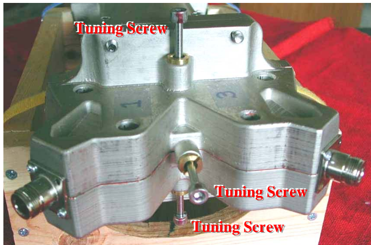
Figure 3.7. Prototype 3 input section with tuning screw locations.
