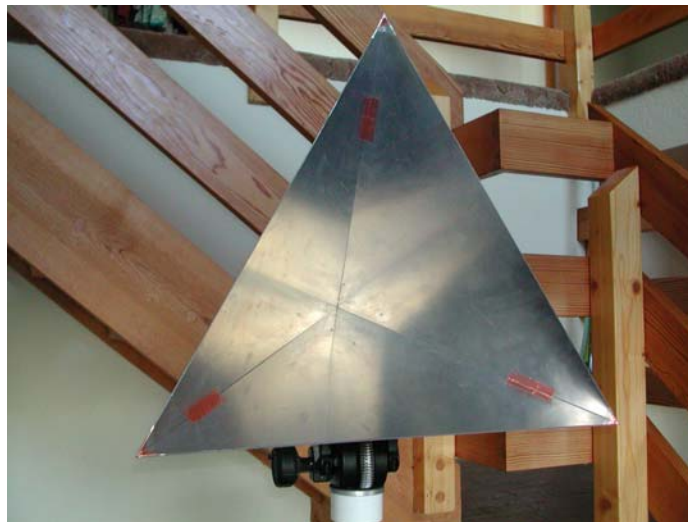
Figure 7.2. Trihedral corner reflector with 60-centimeter sides.
