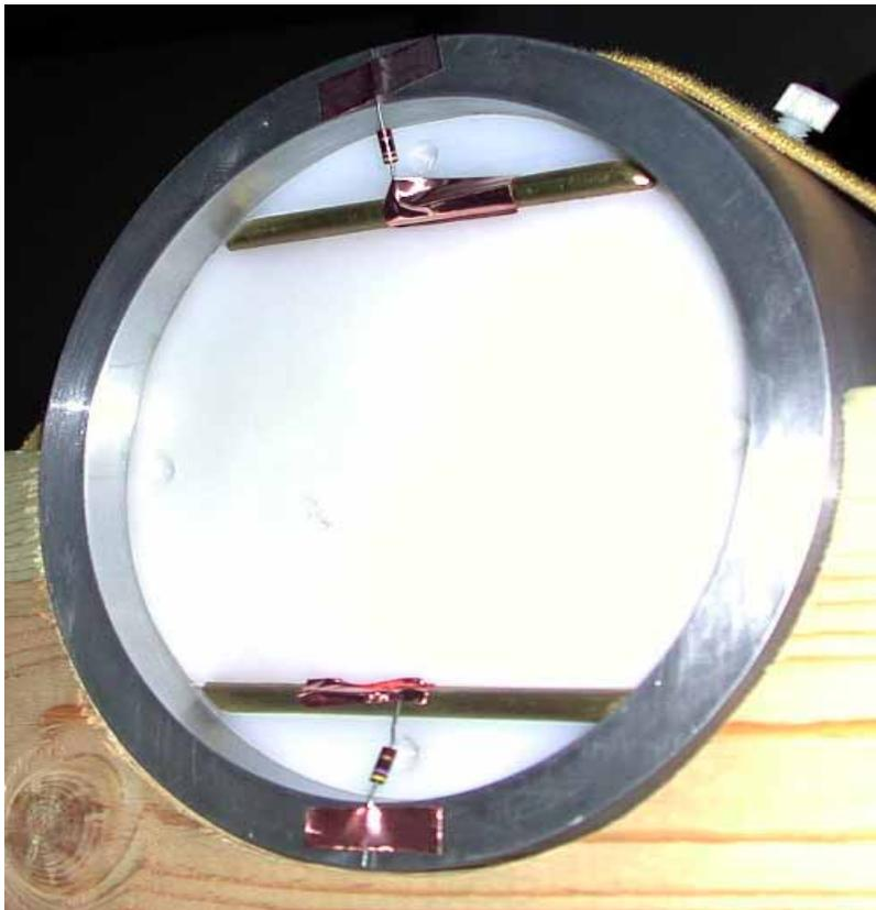
Figure 4.13. Configuration 2, with resistors connected to the shroud.
