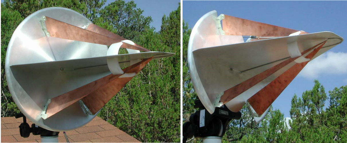
Figure 2.2. IRA-5 (left) and IRA-5b (right) set up for testing.
