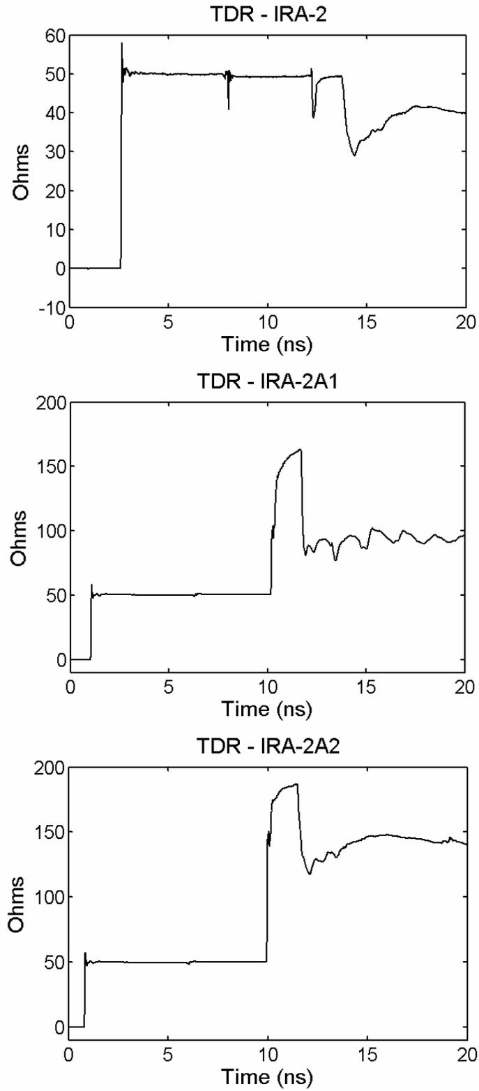
Figure 4.2. TDRs of IRA-2s with standard feed (top), unbalanced feed through center tube (middle), and unbalanced feed along feed arm (bottom).
