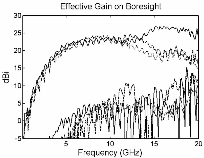
Figure 4.4. Effective gain on boresight including crosspol, for IRA-2s with standard and unbalanced feeds.
