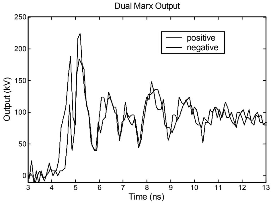
Figure 3.3. Bipolar Marx outputs aligned for maximum.
