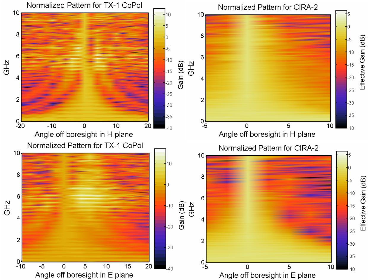
Figure 2.7. Normalized antenna patterns for the TX-1 and CIRA-2.
