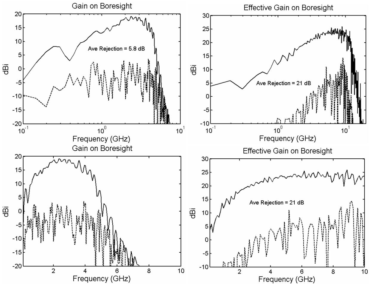
Figure 2.6. Antenna gain and crosspol for the TX-1 (left) and the CIRA-2 antennas, plotted on log (top) and linear (bottom) scales.
