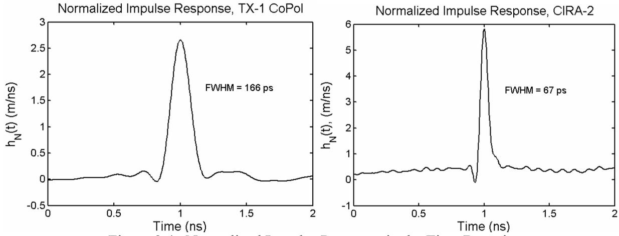
Figure 2.4. Normalized Impulse Response in the Time Domain.
