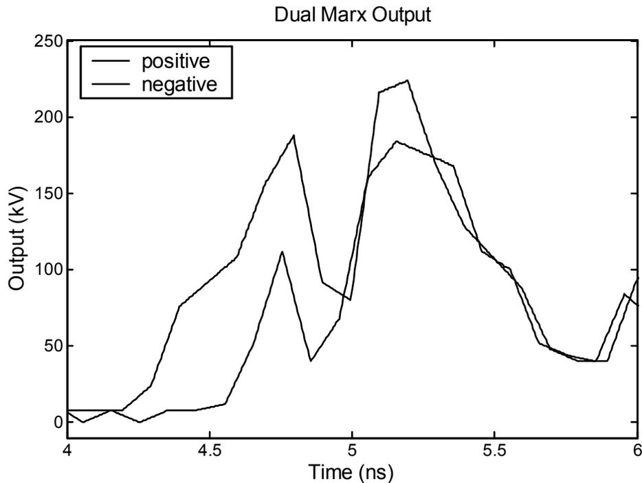
Figure 3.4. Bipolar Marx output expanded to estimate risetime.
