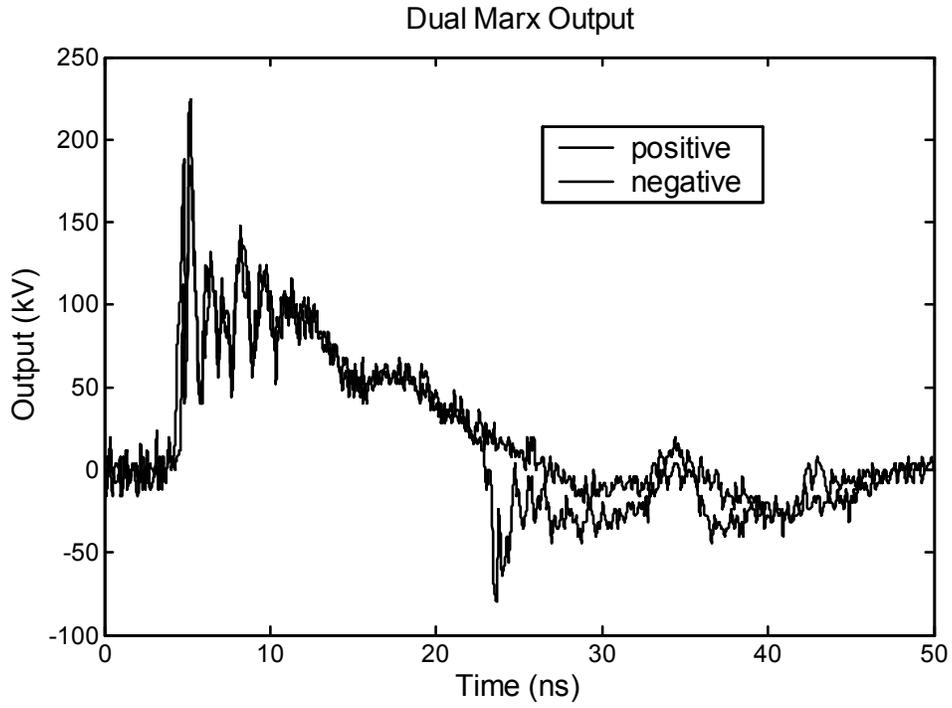
Figure 3.2. Bipolar Marx output.
