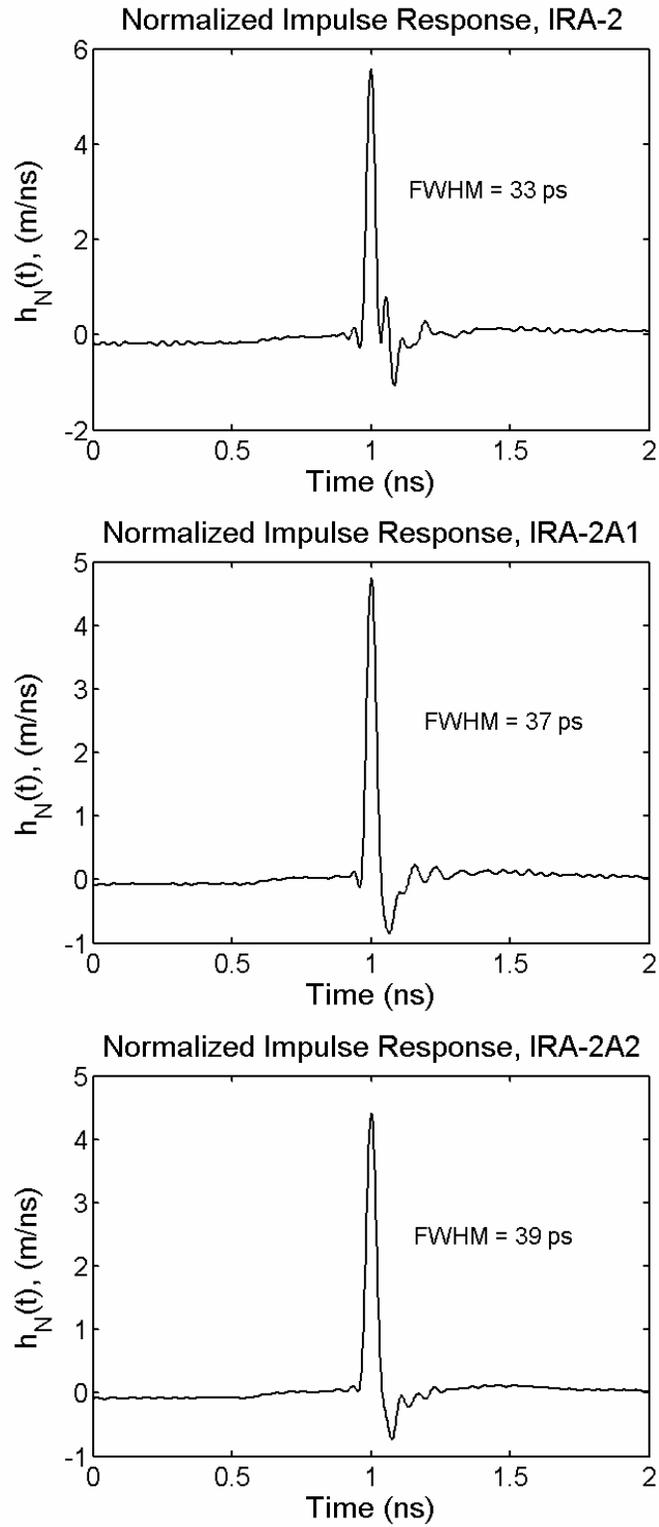
Figure 4.3. Normalized impulse response of IRA-2s with standard feed (top), unbalanced feed through center tube (middle), and unbalanced feed along feed arm (bottom).
