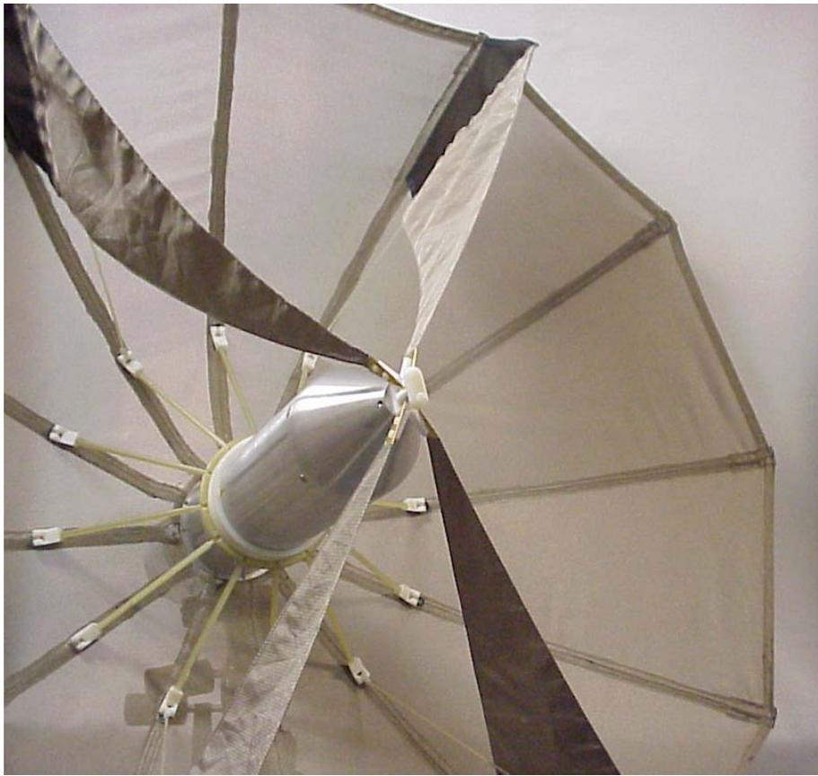
Figure 2.1. TX-1 antenna with large center tube.
