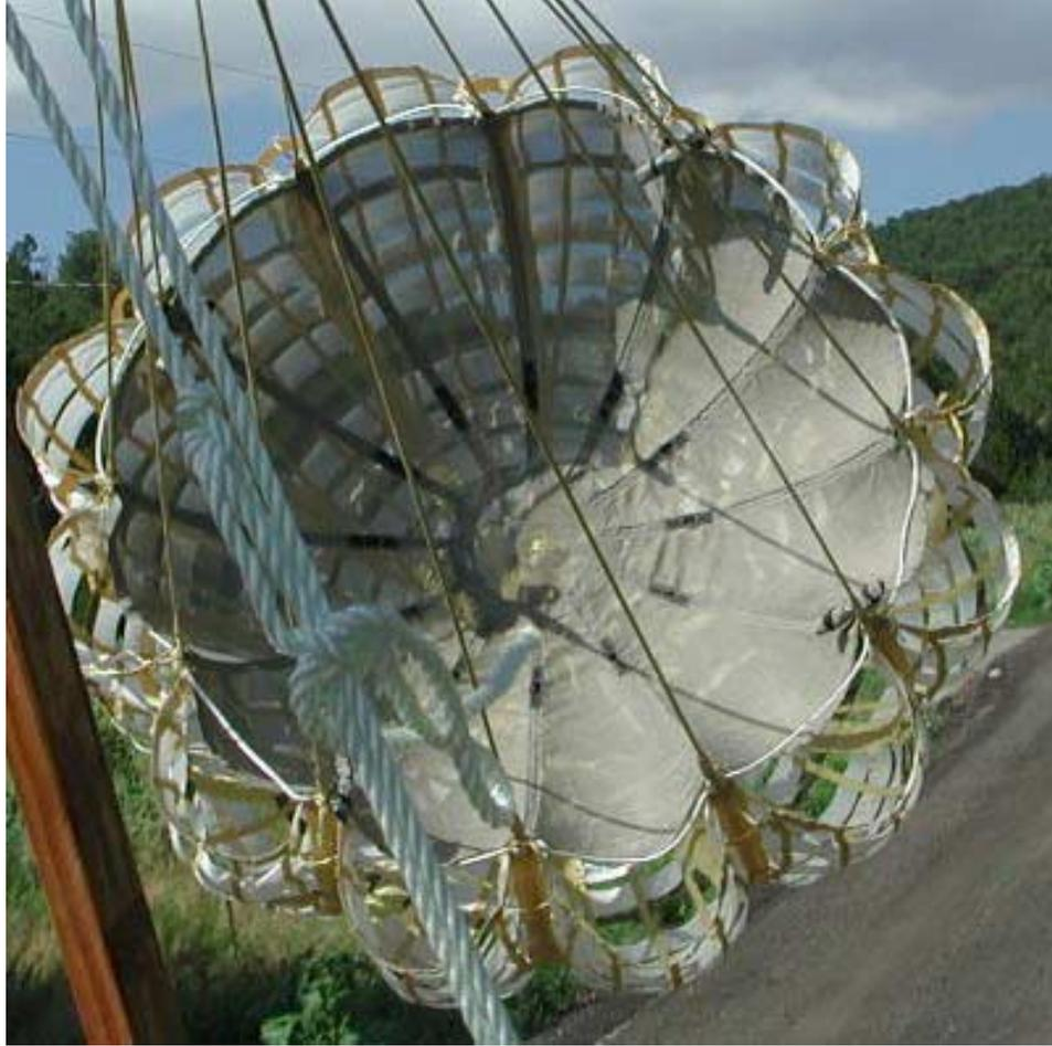
Figure 7.16. Para-IRA inflated during 40 mph (64 kph) tow test.
