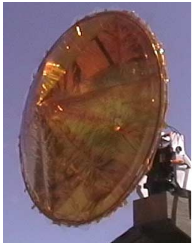
Figure 5.6. Inflated Membrane IRA during RF characterization.
