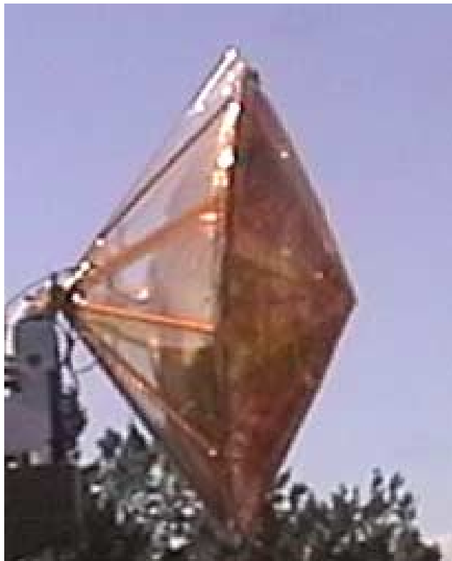
Figure 5.6. Inflated Membrane IRA during RF characterization.
