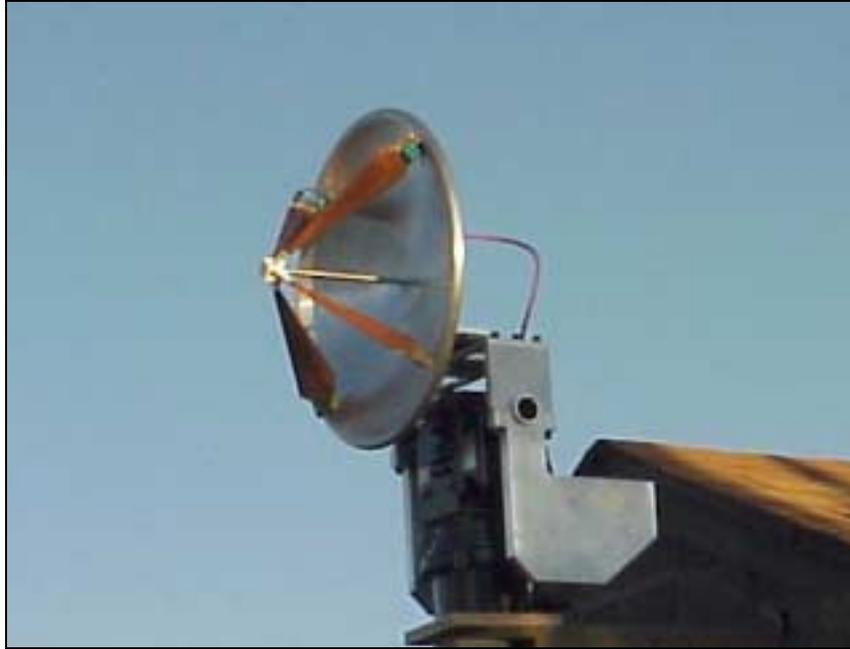
Figure 10. Antenna under test at time domain range. The antenna and AZ-EL positioner assembly is mounted on a raised platform affixed to the front wall of the instrumentation shed.
