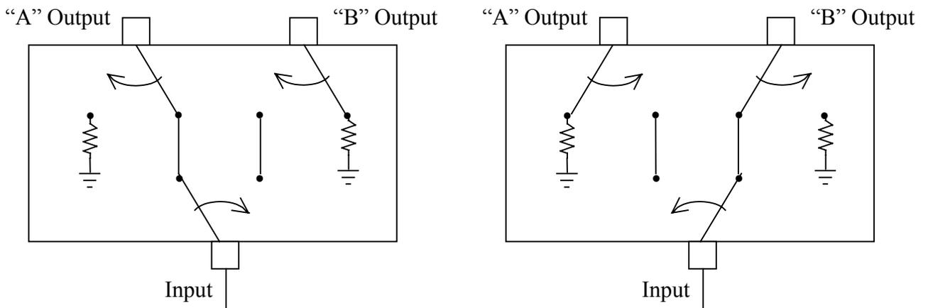
Figure 2.3. Loaded A/B switch, with switch set to “A”(left), and to “B” (right).
