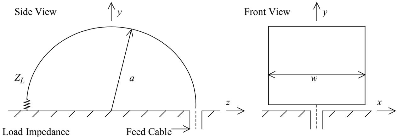
Figure 2.1 Geometry of the BDA.
