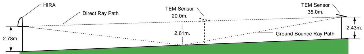
Figure 11. Physical layout of HIRA and TEM sensor for radiated field measurements. The time-of-flight for the ground bounce path is 1.3 ns longer than the direct path when the sensor is 35 m from the HIRA; it is 2.2 ns longer when the sensor is at 20 m.
