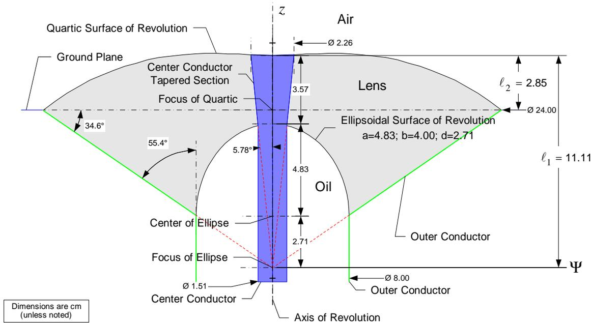
Figure 3. HIRA feed-point lens design. The relative dielectric constant of the lens is 7.0; that of the oil is 2.2.
