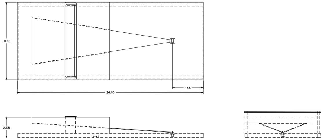
Figure 9. Replicating 50  $\Omega$  TEM sensor. (Dimensions are inches. The original prototype is shown here. We actually used a later version, in which Teflon® posts were used in place of foam to support the conducting strip.)
