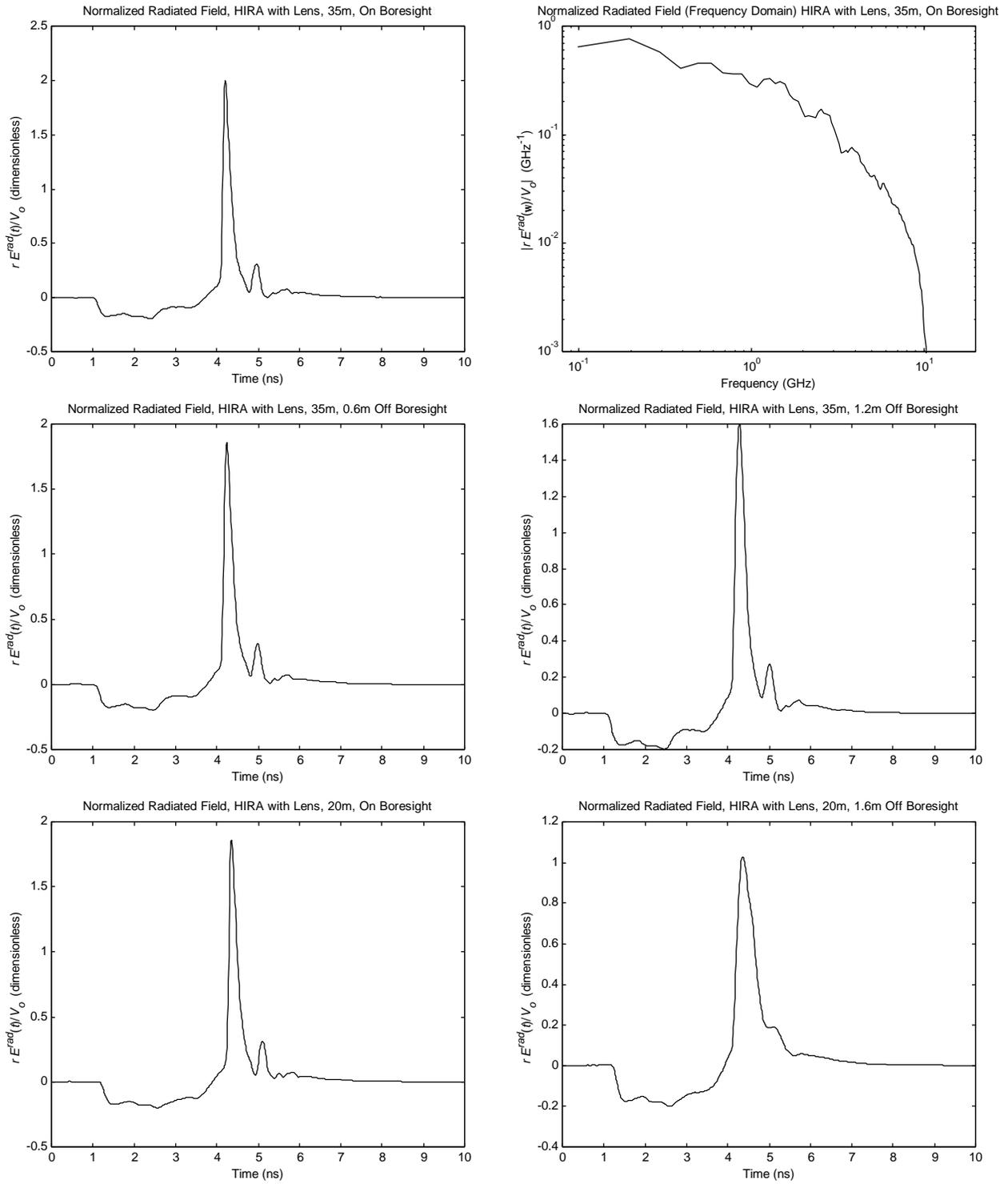
Figure 16. Normalized radiated electric fields at 35 and 20 meter ranges, both on and off boresight. The reference voltage,  $V_o$ , is 25.9 volts.
