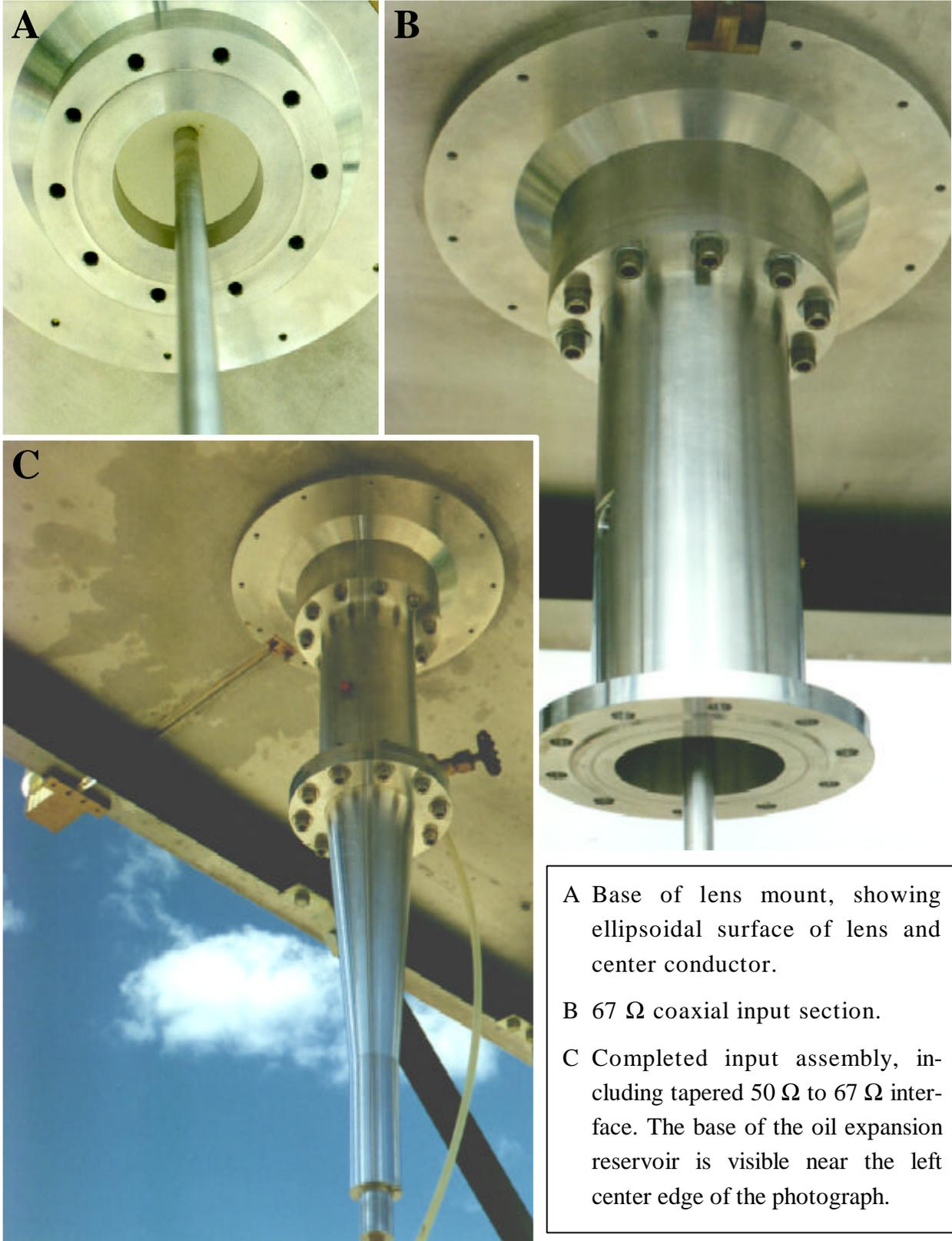
Figure 7. HIRA components located below the ground plane.
