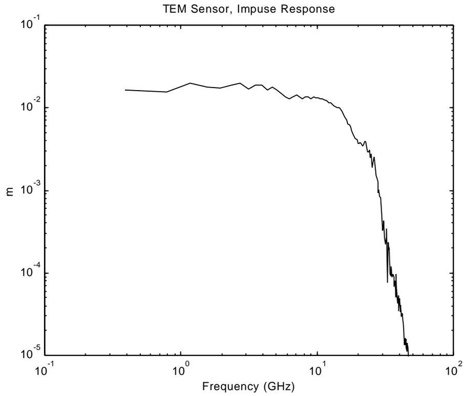
Figure 4.7. TEM sensor impulse response,  $h_{tem}(\omega)$ , in the frequency domain.
