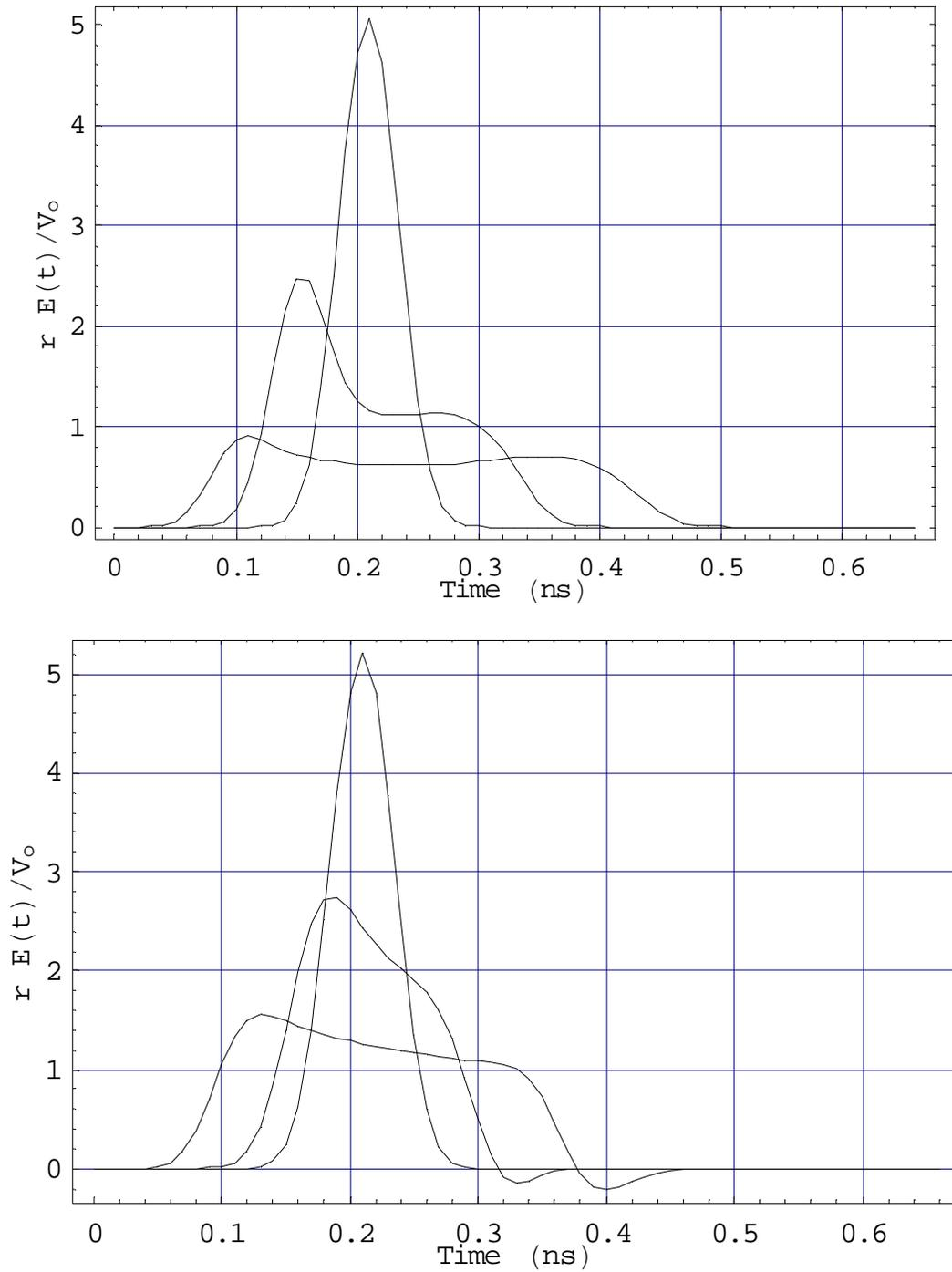
Figure 3.6. MIRA radiated field,  $f_f = 0.85$ , H-plane (top) and E-plane (bottom), at angles of 0, 7.5, and 15 degrees off-boresight.
