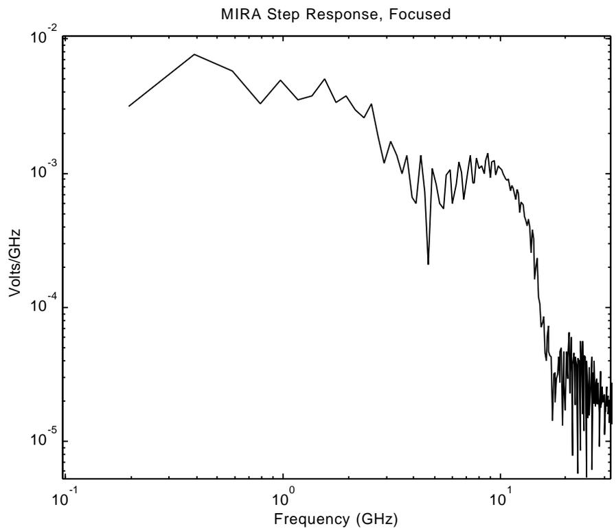
Figure 4.11. Boresight step response of the Multifunction IRA, in the time domain (top) and frequency domain (bottom).
