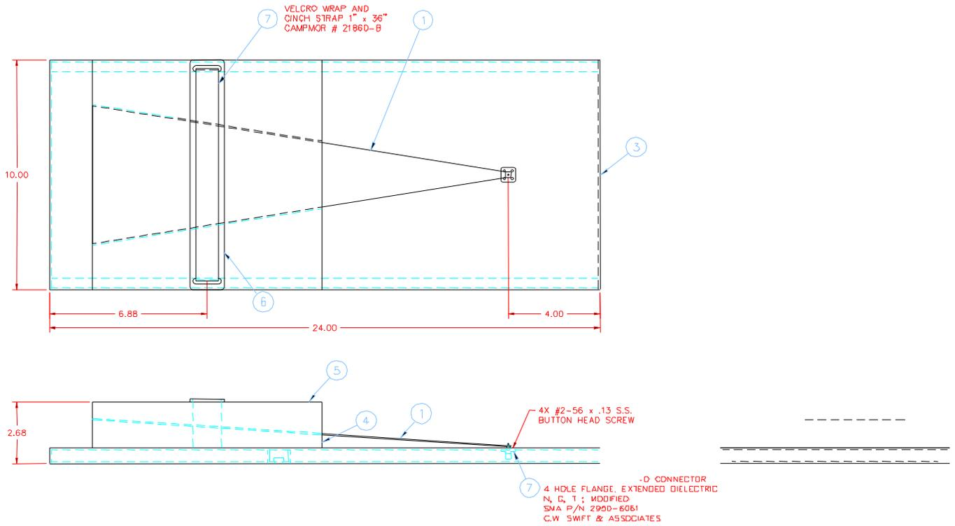
Figure 4.3. TEM Sensor. (Dimensions are inches.)
