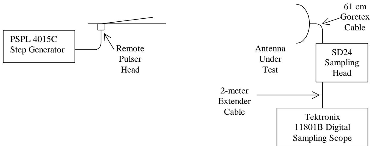
Figure 4.4. Experimental test setup
