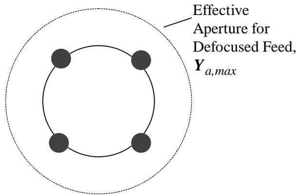
Figure 3.2. The extent of the effective aperture, when a rigid feed arm assembly is pushed closer to the reflector.
