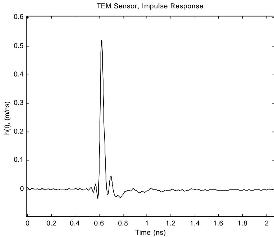
Figure 4.8. TEM sensor impulse response,  $h_{tem}(t)$ , in the time domain.
