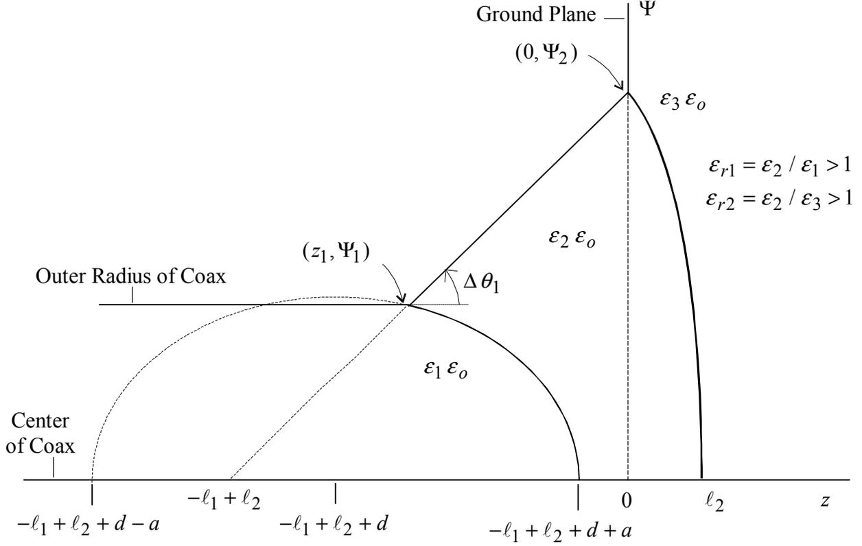
Figure 3.1. Lens design parameters.
