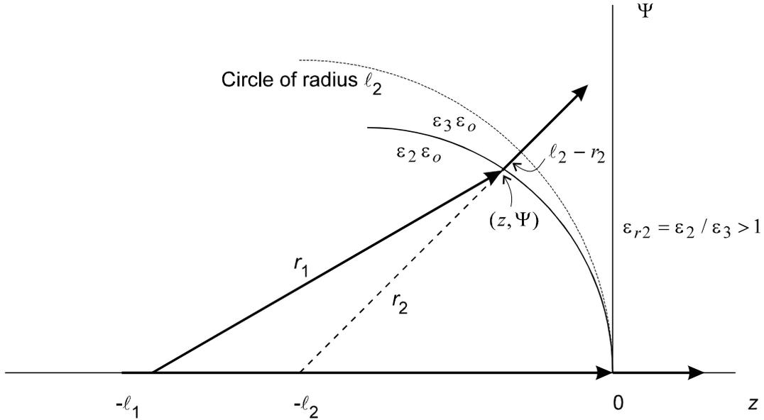
Figure 2.2. Geometry for Interface #2, a quartic surface for converting a spherical wave centered at  $(-l_1, 0)$  to another spherical wave centered at  $(-l_2, 0)$ .
