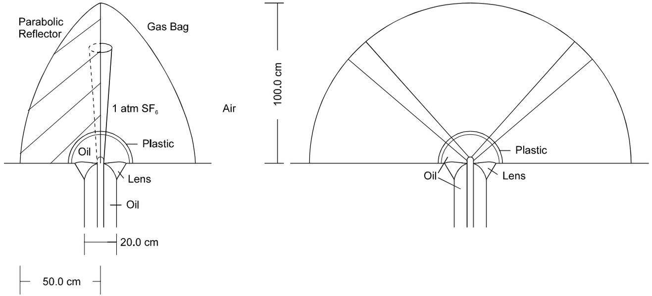
Figure 1.1 A sketch of the Half IRA, shown here with an oil cap.
