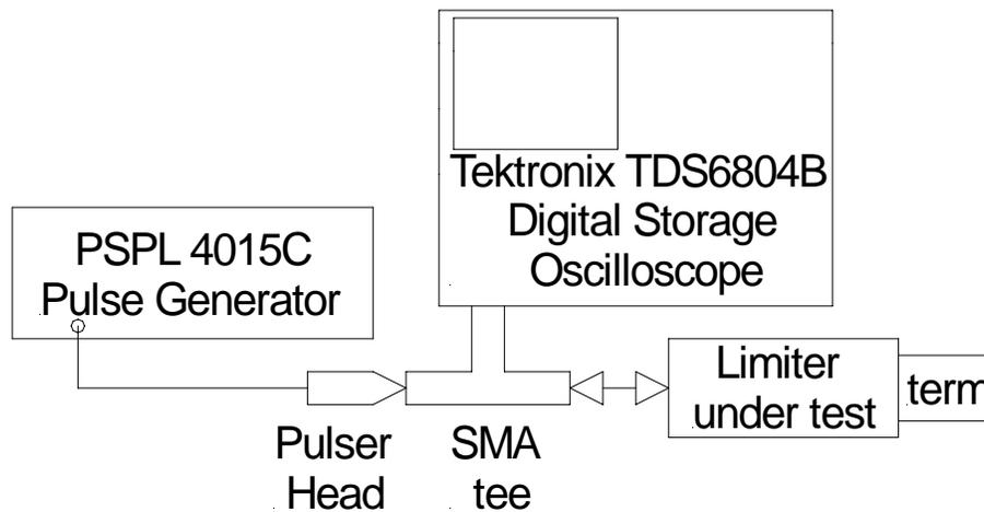
Figure 12. TDR instrumentation.
