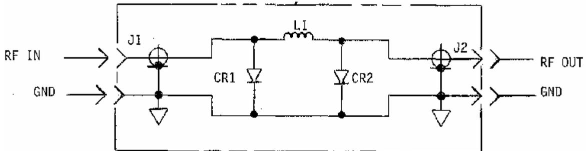
Figure 5. Schematic diagram of the Agilent 11693A limiter.
