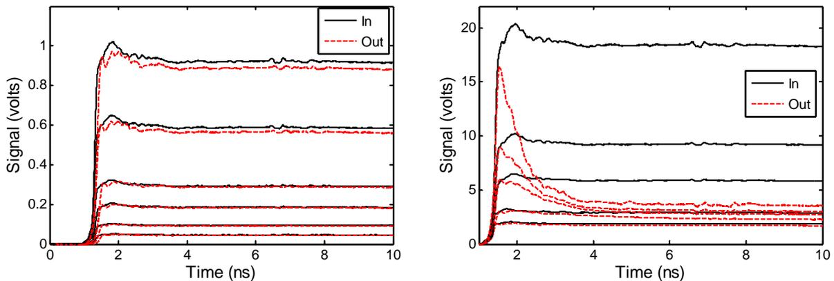
Figure 7. Anritsu 1N50B limiter, negative input, inverted.
