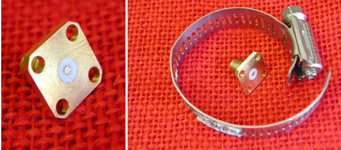
Figure 3. Left: SMA connector modified as a sensor. Right: Sensor and hose clamp.
