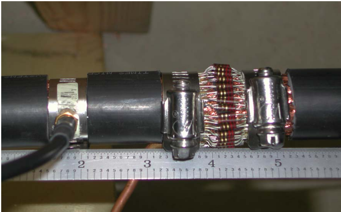
Figure 4. SMA sensor (left) and CVR sensor (right) installed onto the Marx output cable.
