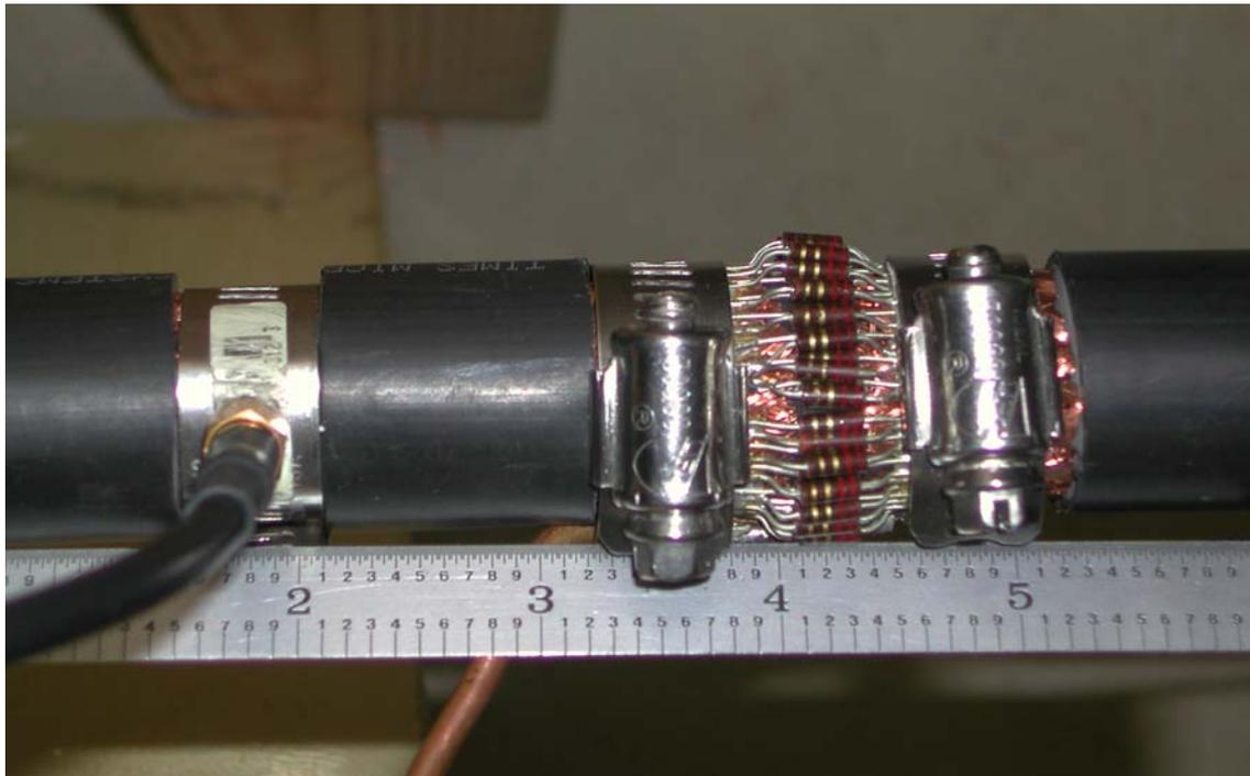
Figure 4. SMA sensor (left) and CVR sensor (right) installed onto the Marx output cable.
