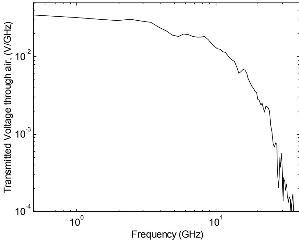
Figure 4.2 Air waveform for the dry sand measurements, time domain (top) and frequency domain (bottom)
