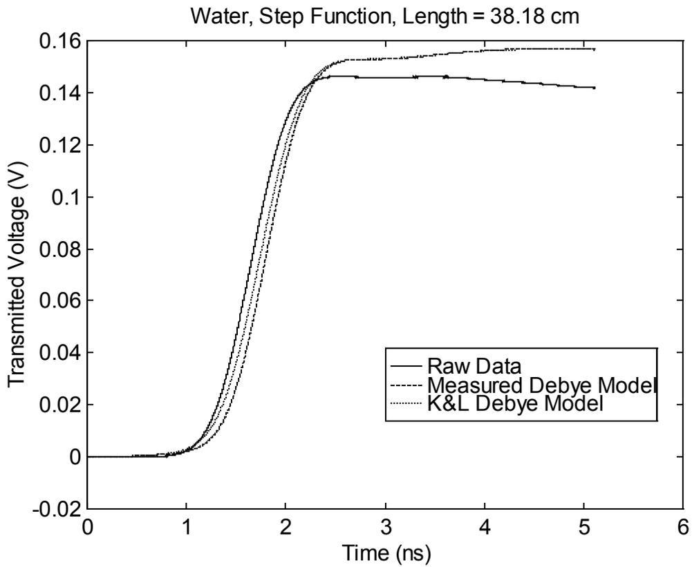
Figure 3.8. Step transmission through 9.52 cm and 38.18 cm water.
