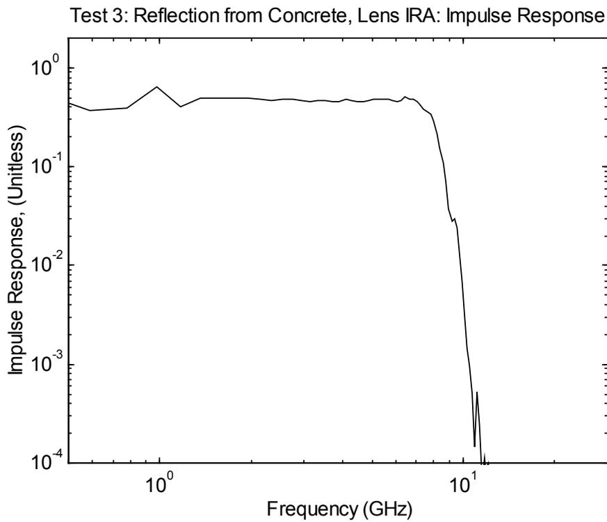
Figure 15.12. Frequency domain impulse response for concrete reflection.
