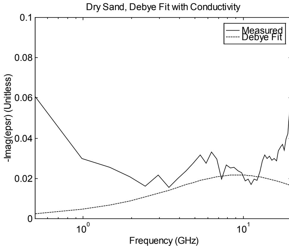
Figure 14.1. Comparison of dry sand dielectric constant to Debye fit, with conductivity.
