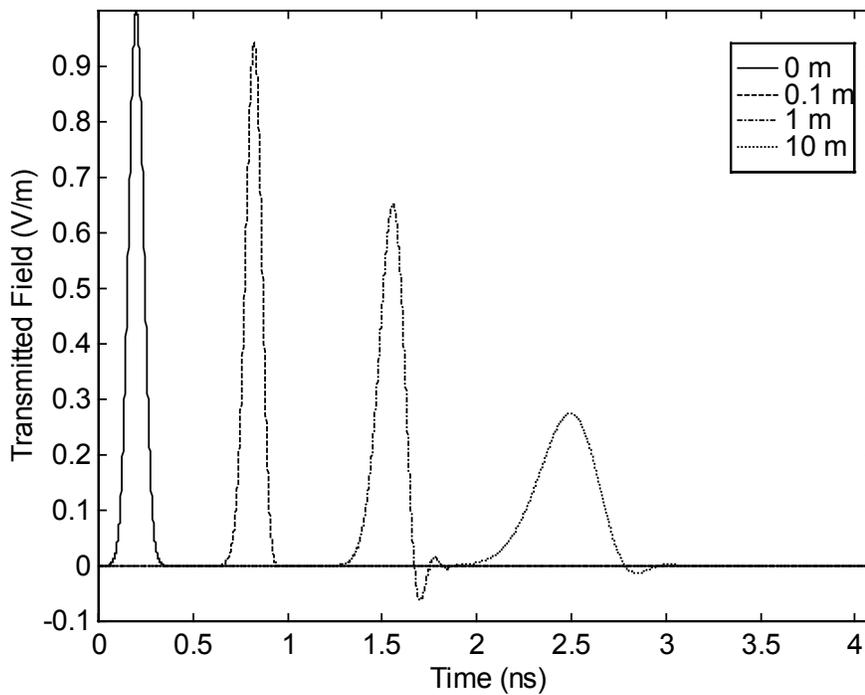
Figure 10.2. The propagated field of the 100 ps pulse at 0, 0.1, 1, and 10 meters. (Starting times shifted for clarity.)
