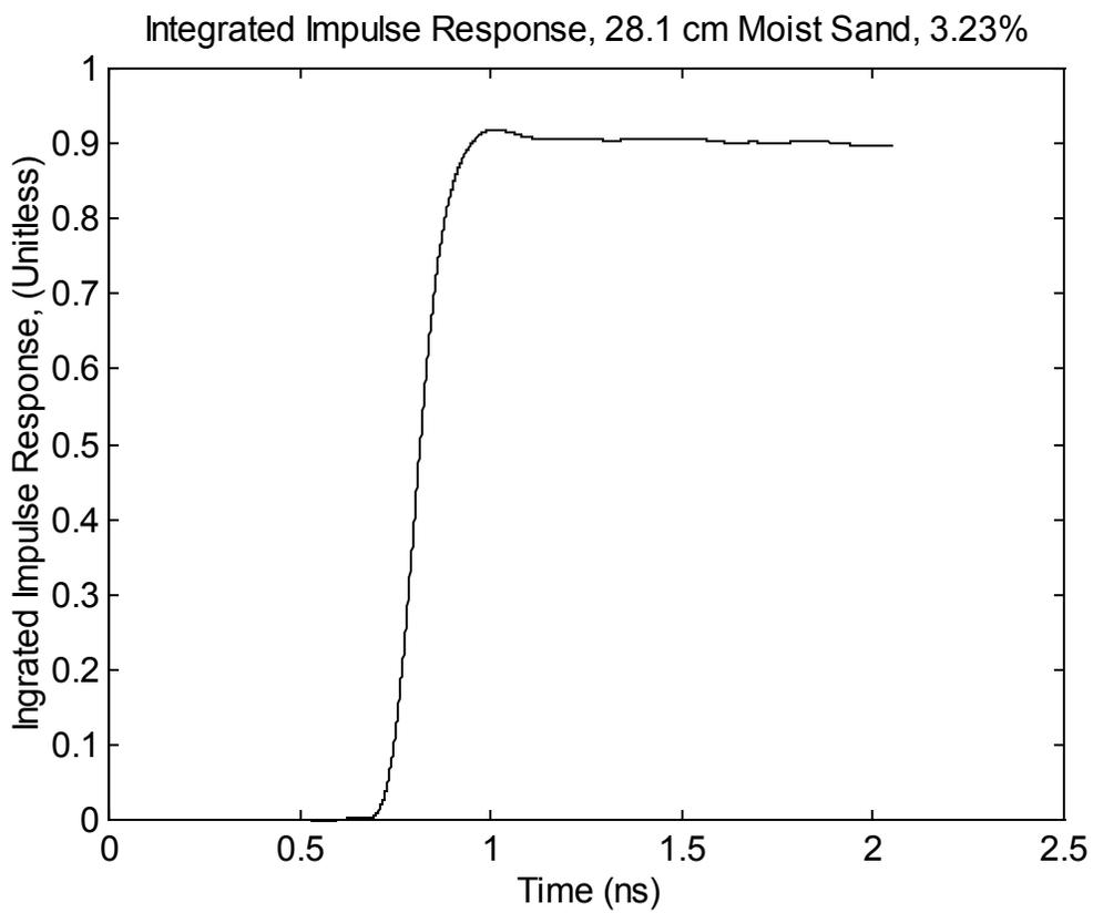
Figure 12.9. The impulse response (top) and its integral (bottom) of 28.1 cm moist sand, 3.23%.
