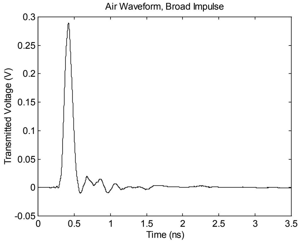
Figure 5.1. Air waveform for the broad impulse.
