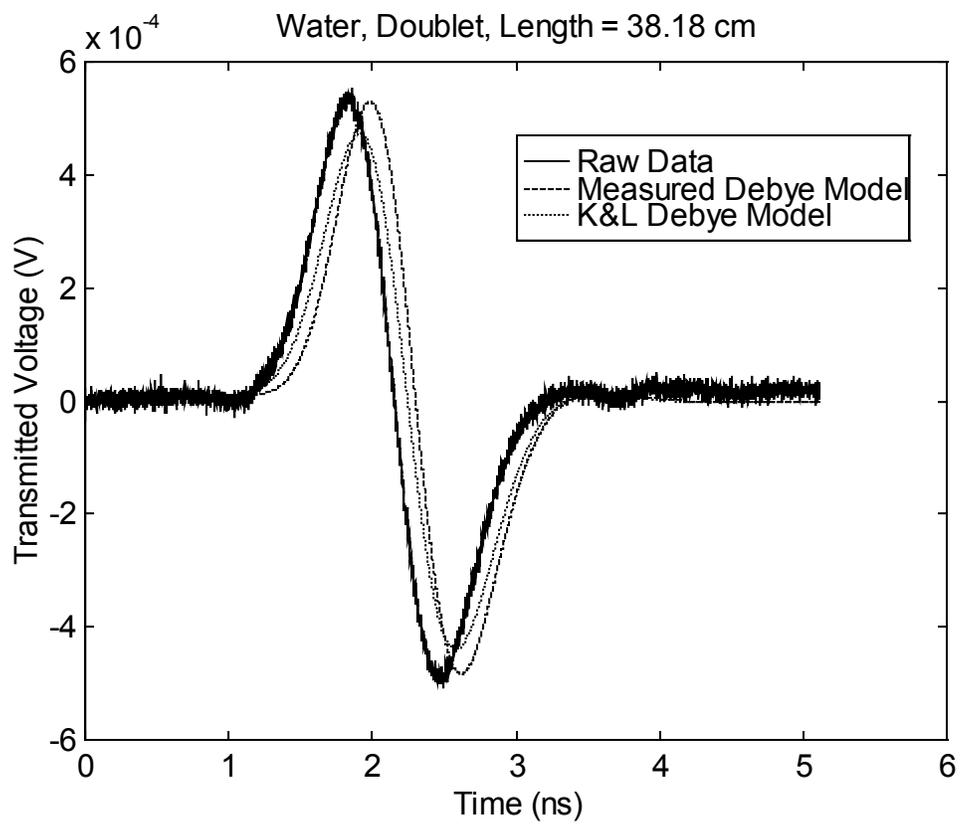
Figure 3.6. Doublet transmission through 9.52 cm and 38.18 cm water.
