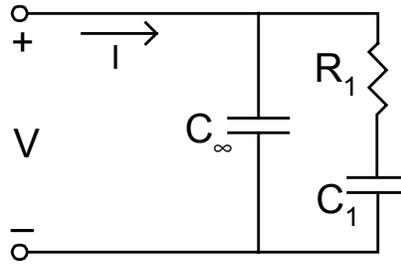
Figure 2.1. Circuit model of the Debye Model.
