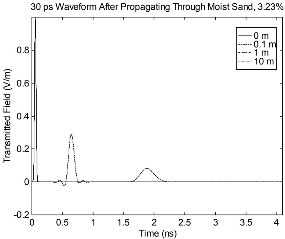
Figure 13.1. The propagated field of the 30 ps pulse at 0, 0.1, 1, and 10 meters, 1.58% top and 3.23% bottom. Note that the 10-meter pulse on the bottom is invisible (Starting times shifted for clarity.)
