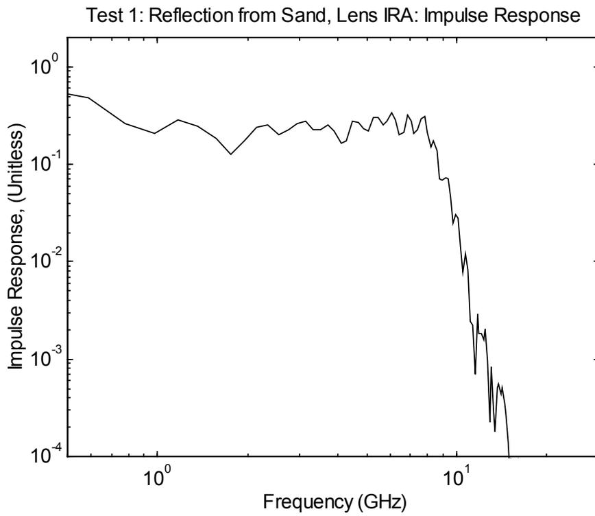
Figure 15.4. Frequency domain impulse response for sand reflection.
