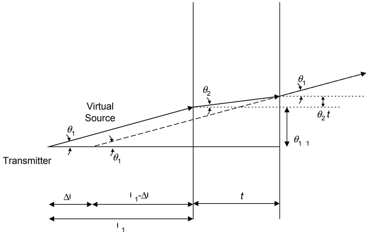
Figure B.2. Layout for determining  $\Delta$ .
