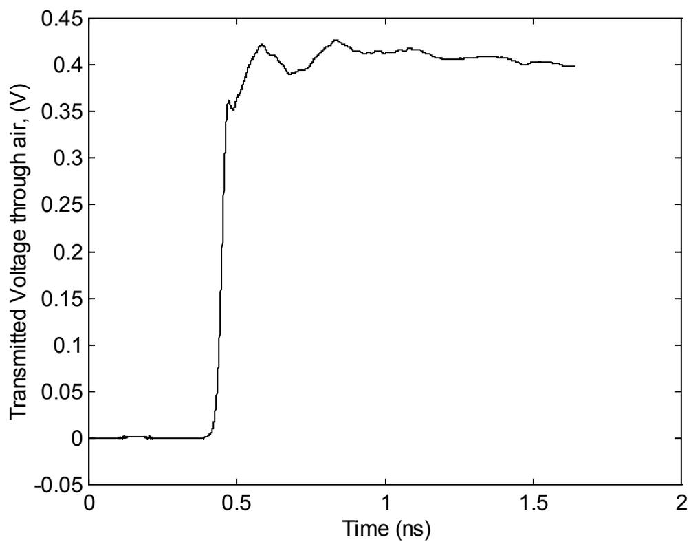
Figure 9.3. Air waveform ( $\epsilon = 0$ ) for the step-function waveshape.
