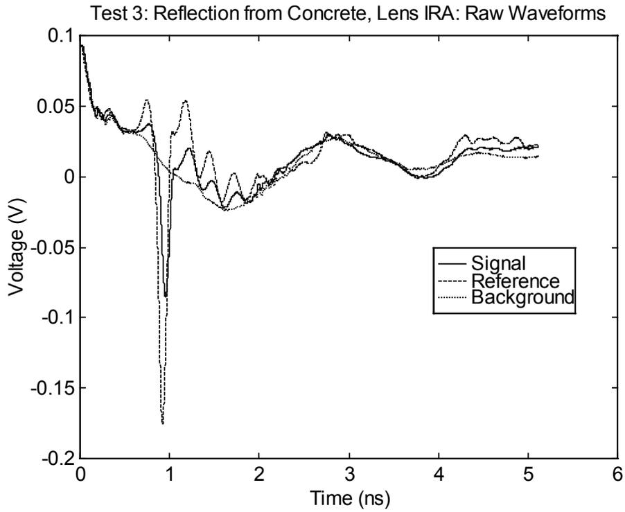
Figure 15.9. Raw data for reflection from concrete.
