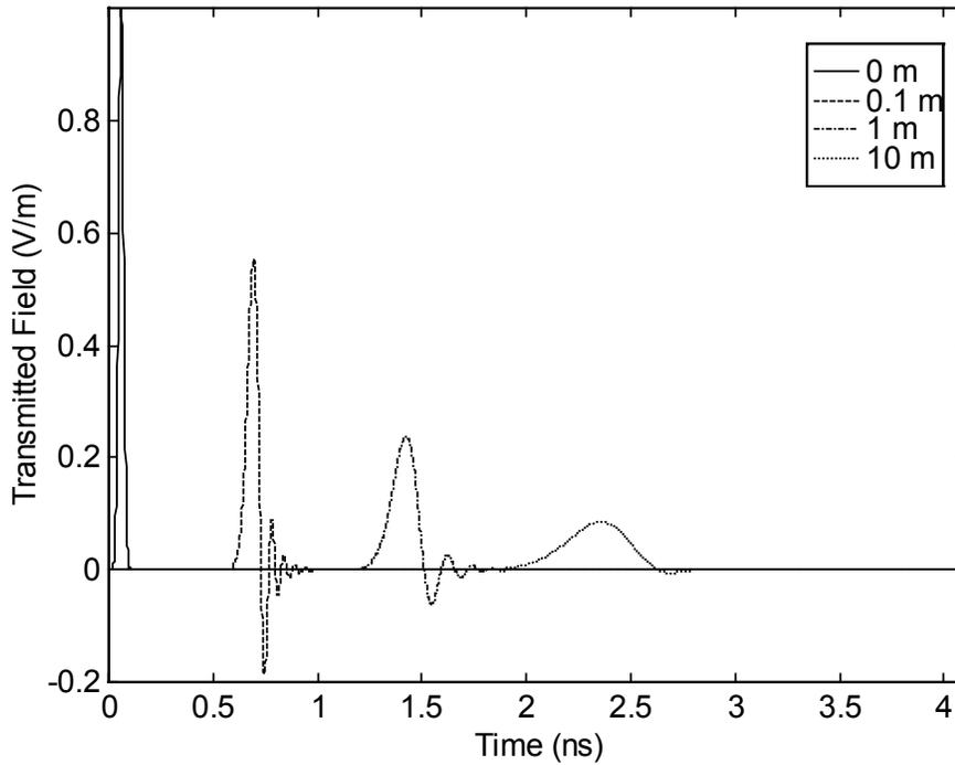
Figure 10.1. The propagated field of the 30 ps pulse at 0, 0.1, 1, and 10 meters. (Starting times shifted for clarity.)
