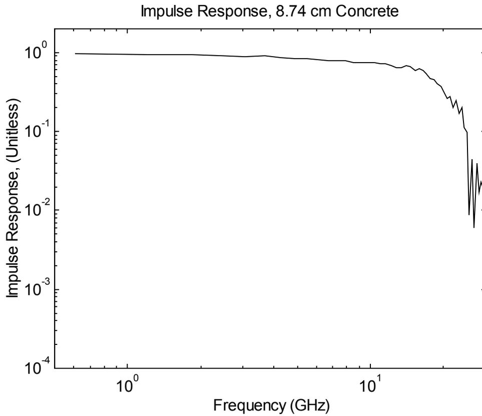
Figure 8.4. The impulse response of 8.74 cm of concrete.
