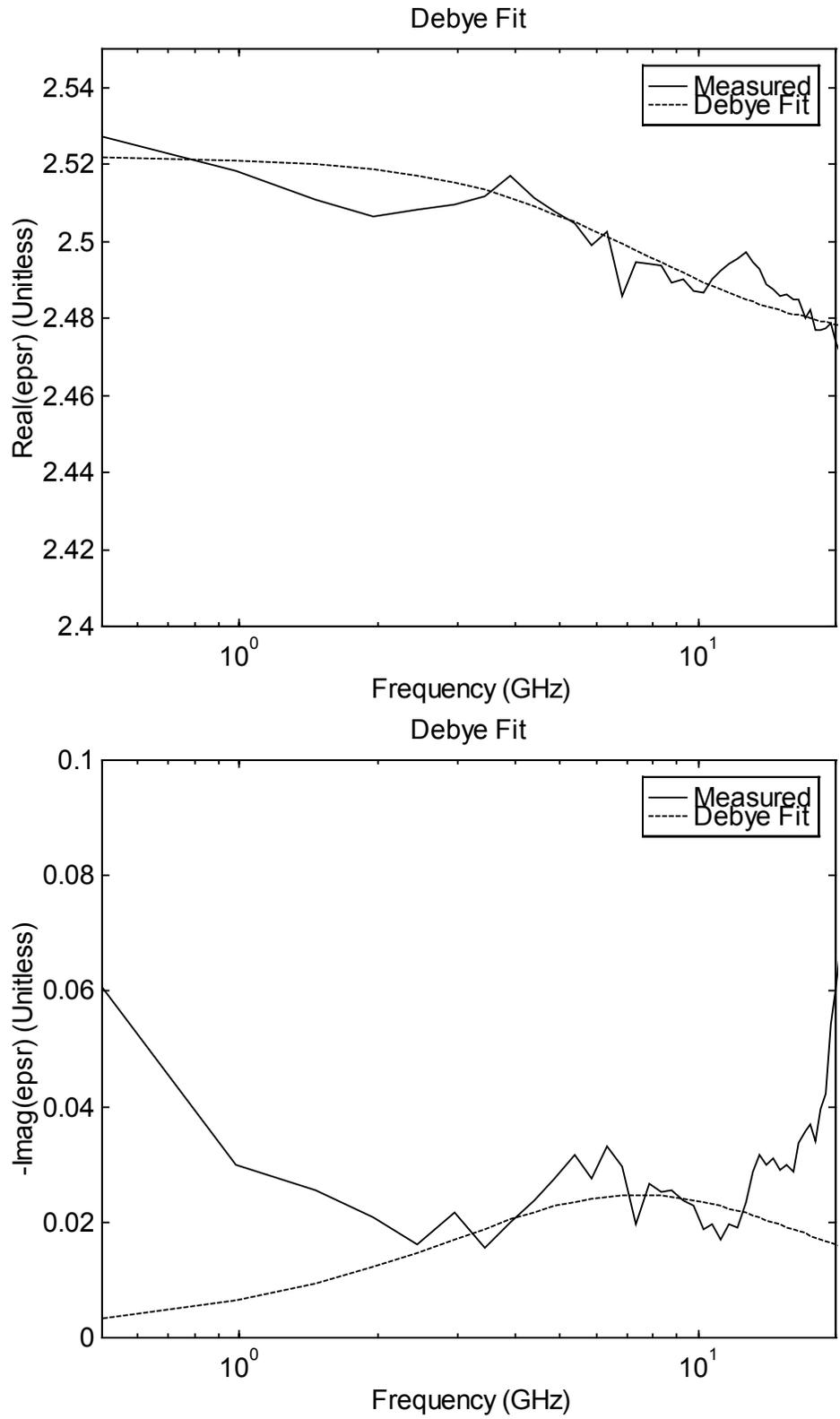
Figure 4.6. Measured dielectric constant of dry sand, and the Debye fit, real and imaginary parts.
