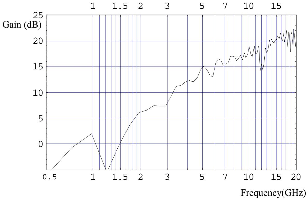
Figure A.1. Gain of the nine-inch reflector IRA.
