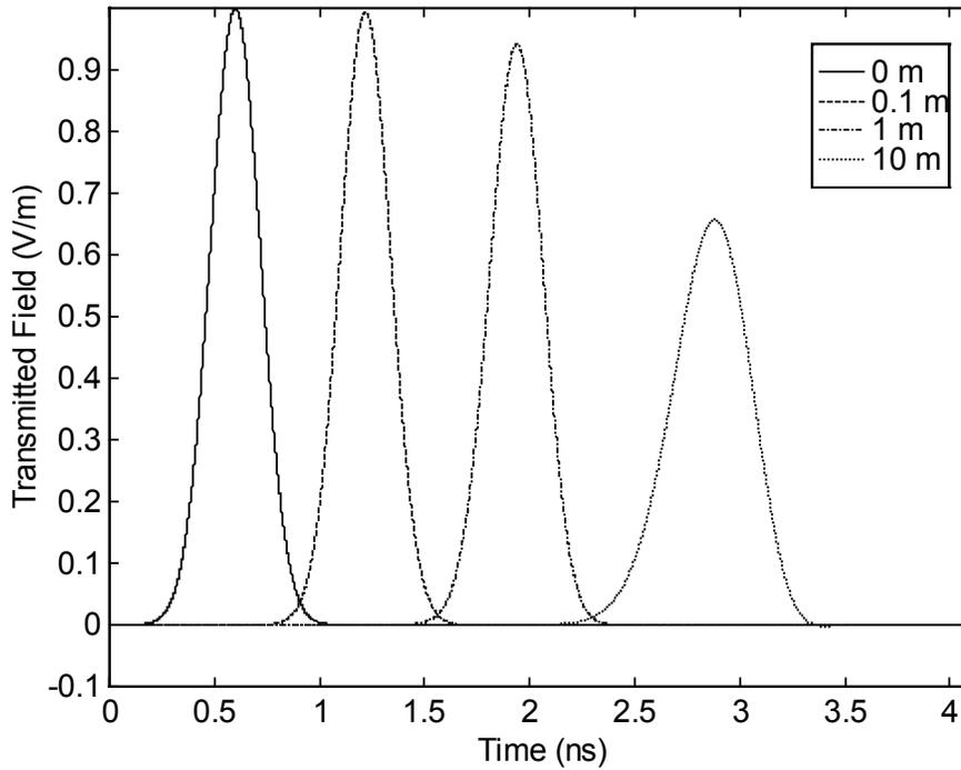
Figure 10.3. The propagated field of the 300 ps pulse at 0, 0.1, 1, and 10 meters. (Starting times shifted for clarity.)
