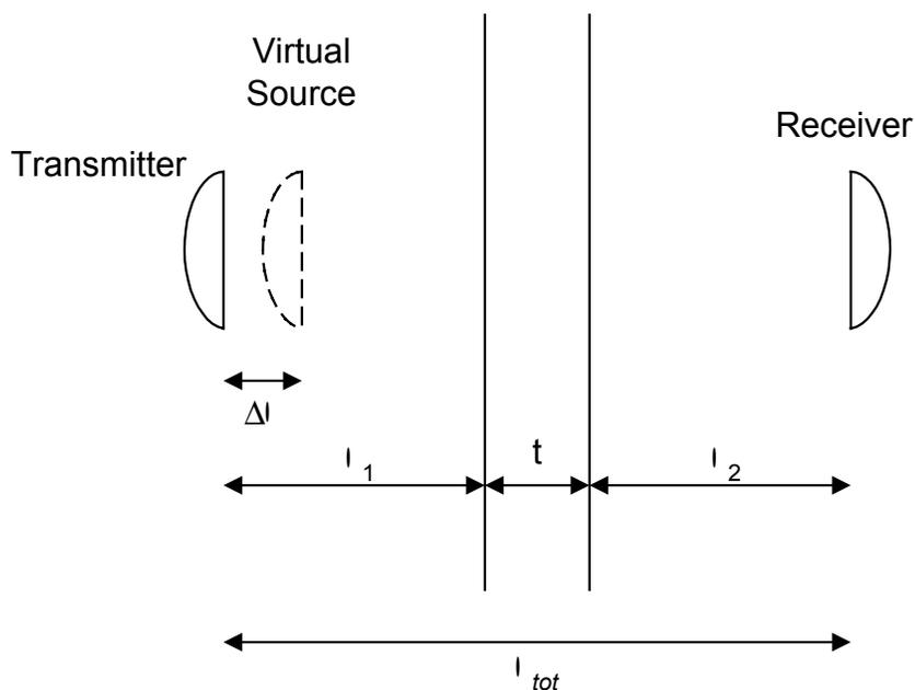
Figure B.1. Two antennas on either side of a dielectric slab, with the virtual source.
