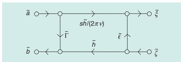
**FIGURE 2.** A signal-flow graph of the antenna equation, on boresight, for single polarization.
