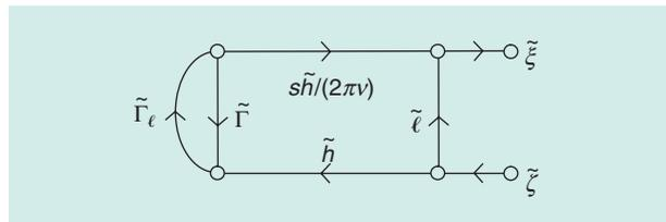
FIGURE 7. The radar scattering from an antenna with an arbitrary load.
