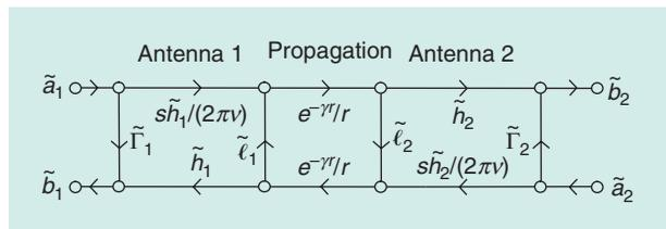
FIGURE 8. Two antennas with a propagation term.
