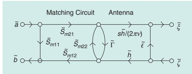
FIGURE 6. An antenna with a matching circuit.
