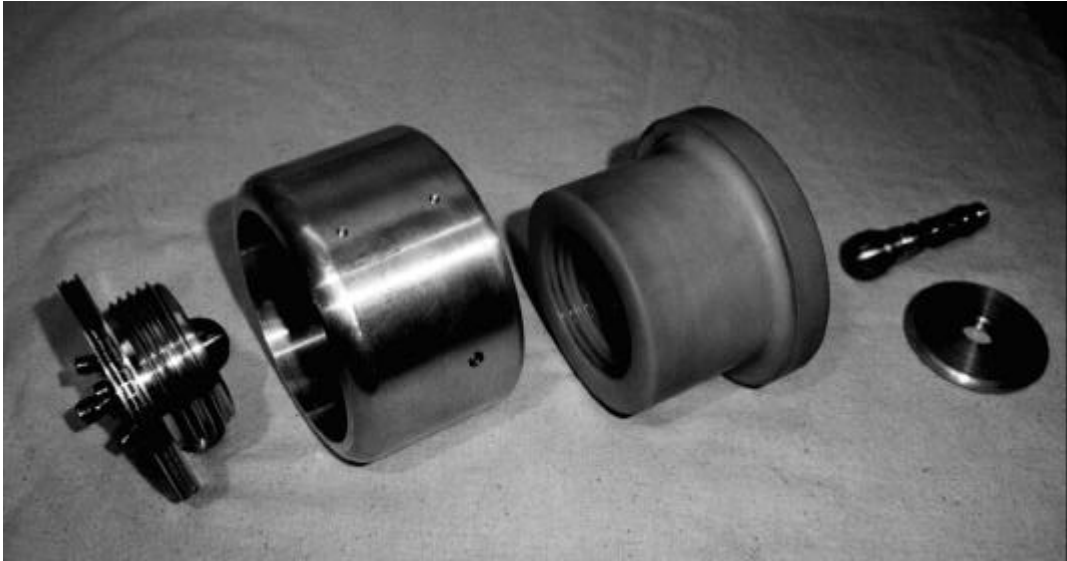
Figure 3.4. Photograph of partially assembled switch.
