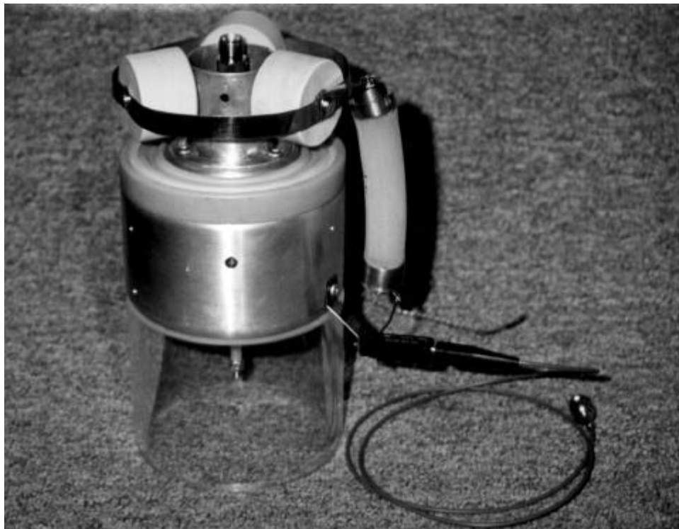
Figure 4.3. Assembled High-Voltage, High-Pressure Switch
