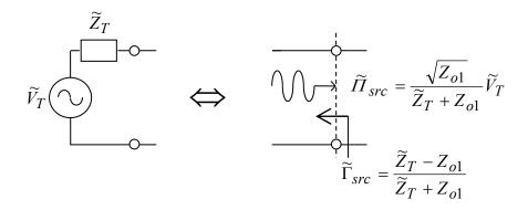
Figure 7.2. The relationship between a Thévenin equivalent source (left) and a power wave source (right) at a port with reference impedance  $Z_{o1}$ .
