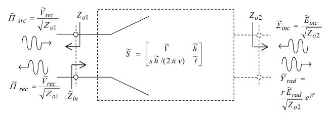
Figure 6.1. The Generalized Antenna Scattering Matrix (GASM), on boresight, for dominant polarization.
