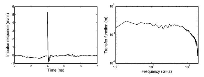
Figure 9.1. Impulse response (left) and transfer function (right) of the IRA-3Q.
