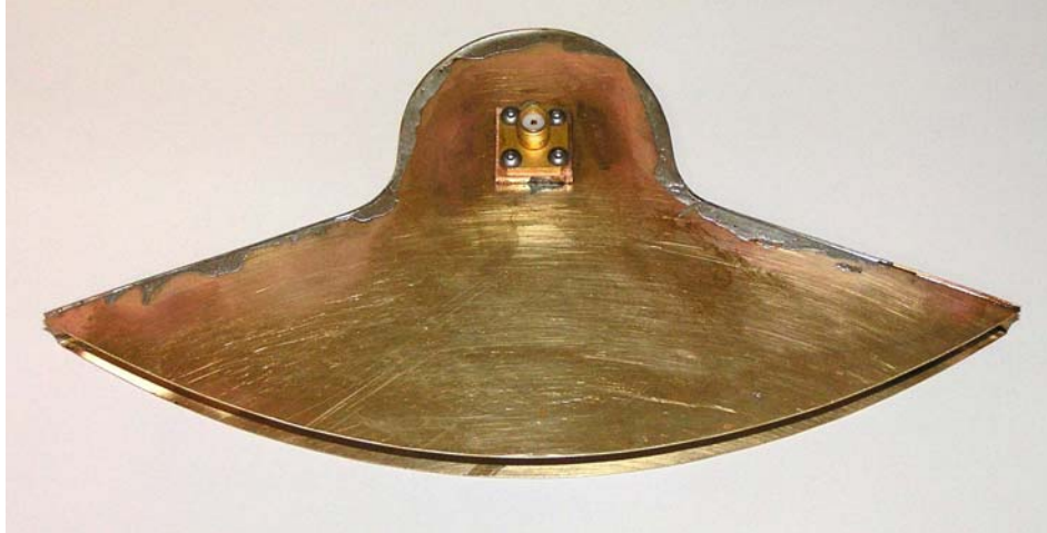
Figure 3.3. Bottom view of the FH-1-FS showing the SMA connector at the feed point.
