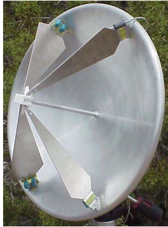
Figure 4.2. IRA-2 with feed arms at \pm 30^\circ .
