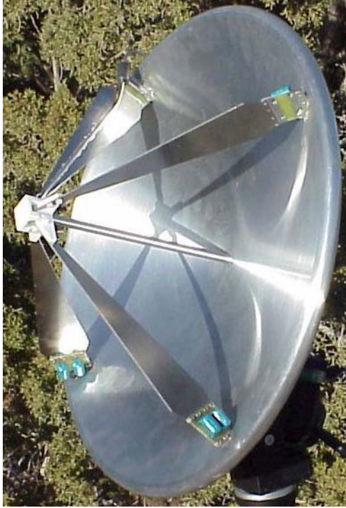
Figure 4.1. IRA-1 with feed arms at \pm 45^\circ .
