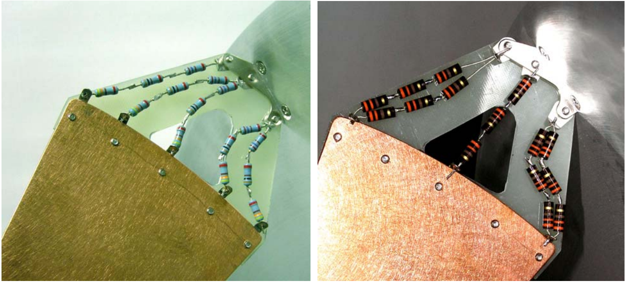
Figure 6.1. Resistor configuration of the IRA-2B, with metal-film resistors (left) and the IRA-2C, with carbon-composition resistors (right).
