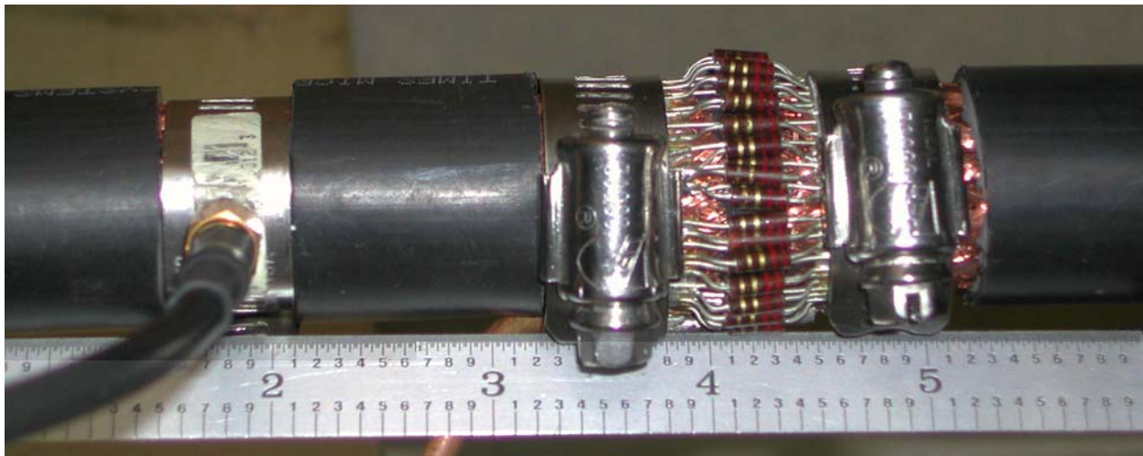
Figure 3.4. SMA sensor (left) and CVR sensor (right) installed onto the Marx output cable.
