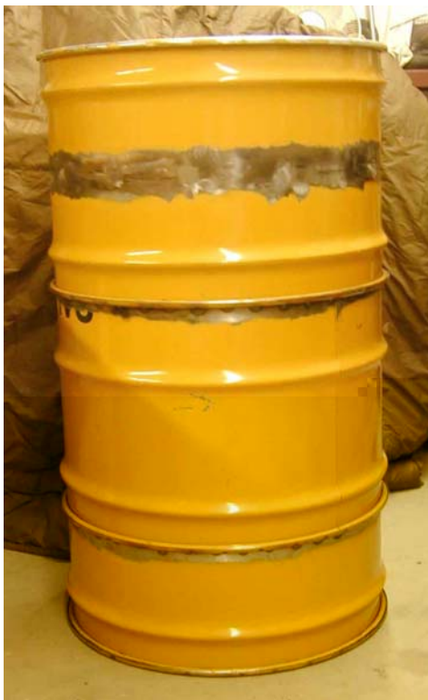
Figure 3.2. High voltage RF containment chamber.
