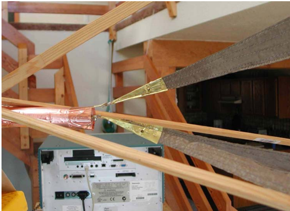
Figure 2.4. Adaptor configured coaxially.
