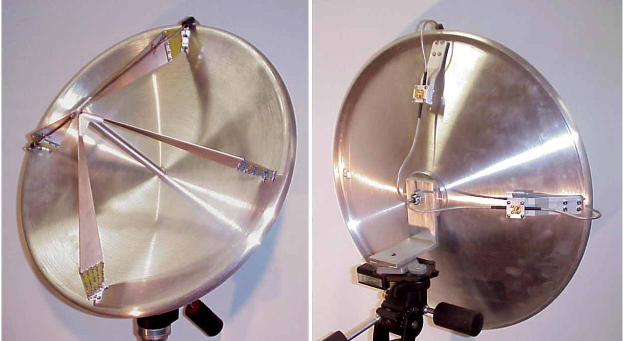
Figure 1. IRA-1D, front and back showing dual polarization feeds.
