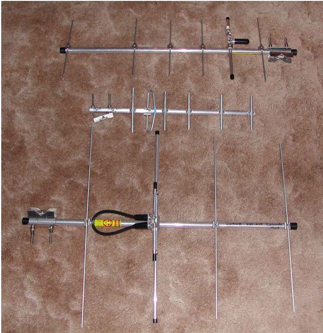
Figure 7.1. Test antennas – from top to bottom: Cushcraft A4496S (6-element yagi), M 2 Model 900-930-6W (6-element folded dipole), and Cushcraft 224WB (4-element Yagi).
