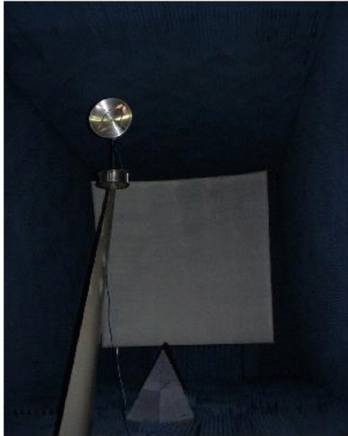
Figure 4.1. The IRA antenna under going tests in MRC's anechoic chamber.
