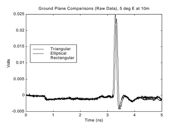
Figure 2.17. Comparision of Ground Plane Configurations.
