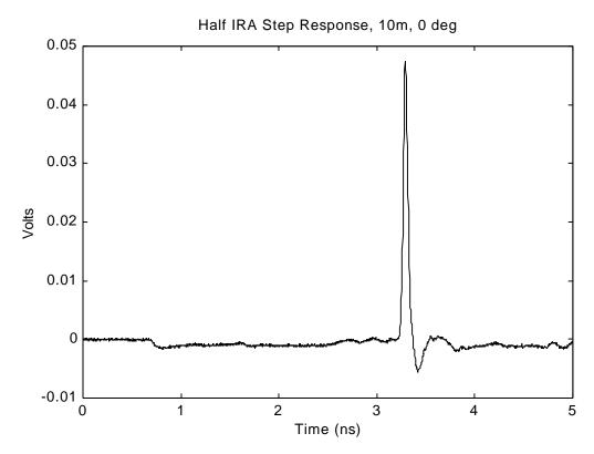
Figure 2.9. Measured Voltage on Boresight at 10 m.
