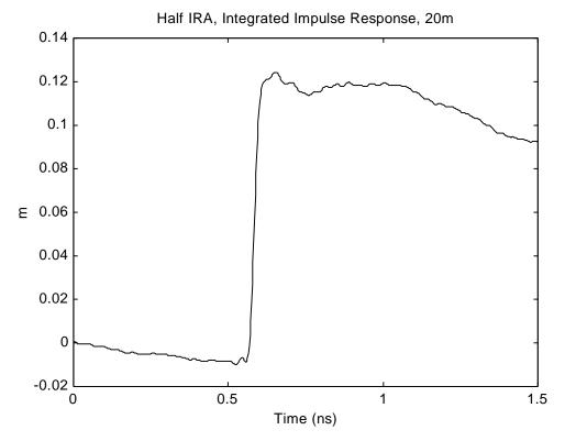
Figure 2.3  $h_{HIRA}(t)$  dt, Effective height 0.13m.
