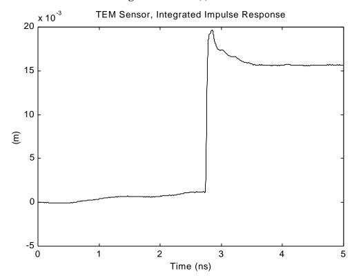
Figure 1.4.  $\hat{o}h_{TEM}(t)$  dt, Effective Height »17mm.
