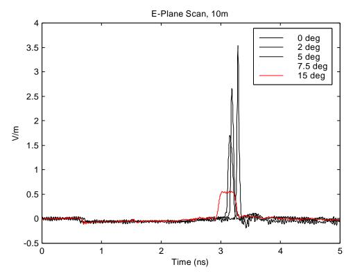
Figure 2.13. E Plane Scan (skyward) at 10 m.
