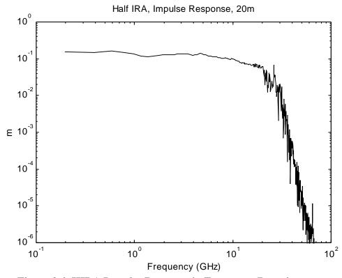
Figure 2.4 HIRA Impulse Response in Frequency Domain.
