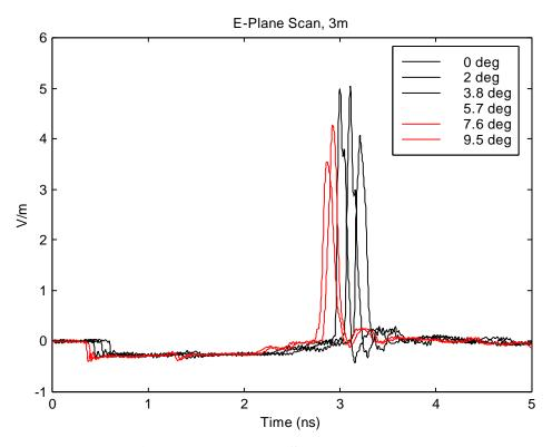
Figure 2.8. E Plane Scan at 3 m.
