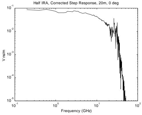
Figure 2.21. HIRA Corrected Step Response on Boresight at 20 m.
