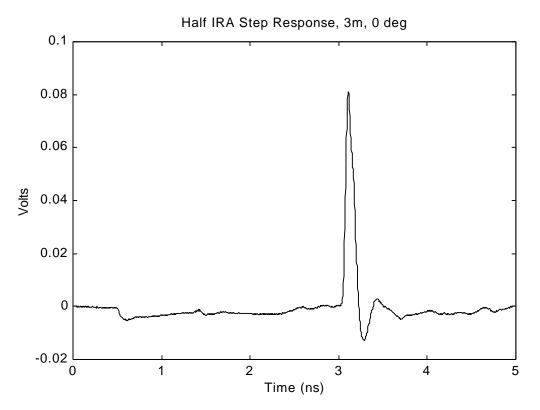
Figure 2.5. Measured Voltage on Boresight at 3 m.
