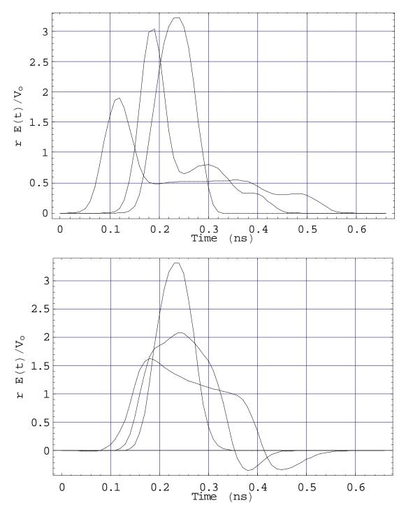
Figure 3.7. MIRA radiated field,  $f_f$  = 0.7, H-plane (top) and E-plane (bottom), at angles of 0, 7.5, and 15 degrees off-boresight.
