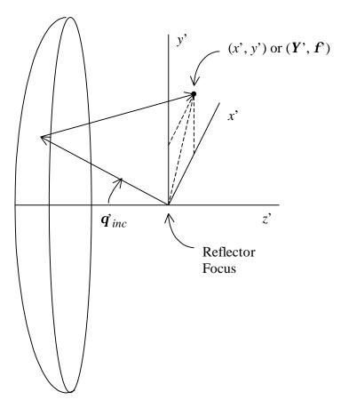
Figure 3.3. The ray trace from the focus to a point in the aperture plane.
