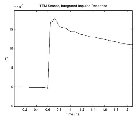
Figure 4.9. Integral of the TEM sensor impulse response.
