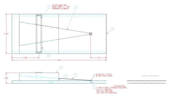
Figure 4.3. TEM Sensor. (Dimensions are inches.)
