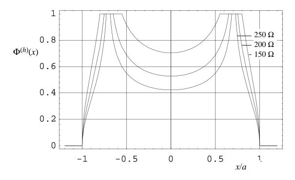
Figure 2.4. The normalized potential function of a 4-wire aperture,  $\Phi^{(h)}(x)$ , plotted for a few different four-wire feed impedances.
