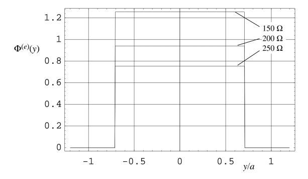
Figure 2.5. The normalized potential function of a 4-wire aperture,  $\Phi^{(e)}(y)$ , plotted for a few different four-wire feed impedances.
