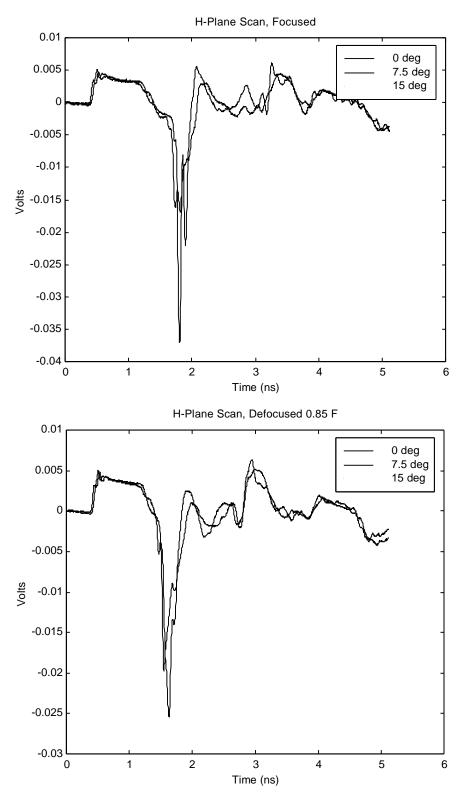
Figure 4.12. Antenna response for MIRA with  $f_f = 1.0$  (top), and  $f_f = 0.85$  (bottom). Antenna responses are for 0, 7.5, and 15 degrees off boresight in the H-plane. The results for  $f_f = 0.70$  are on the next page.
