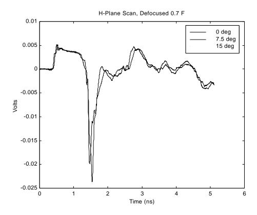
Figure 4.12 (cont'd). Antenna response for MIRA with  $f_f = 0.70$ . Antenna responses are for 0, 7.5, and 15 degrees off boresight in the H-plane.
