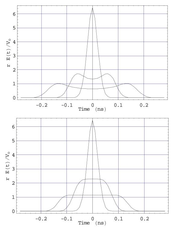
Figure 3.5. MIRA radiated field,  $f_f$  = 1.0 (in focus), H-plane (top) and E-plane (bottom), at angles of 0, 7.5, and 15 degrees off-boresight.
