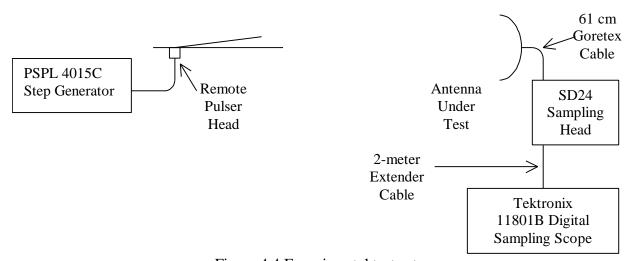
Figure 4.4.Experimental test setup
