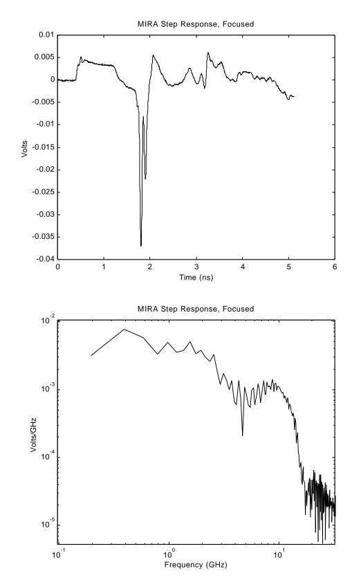
Figure 4.11. Boresight step response of the Multifunction IRA, in the time domain (top) and frequency domain (bottom).
