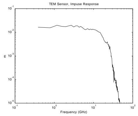
Figure 4.7. TEM sensor impulse response,  $h_{tem}(\mathbf{w})$ , in the frequency domain.
