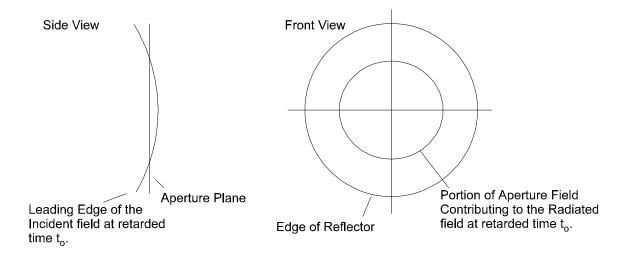
Figure 3.1. Illustration of how a defocused aperture is filled gradually by the incident field (left). The portion of the aperture plane contributing to the aperture field is shown on the right.
