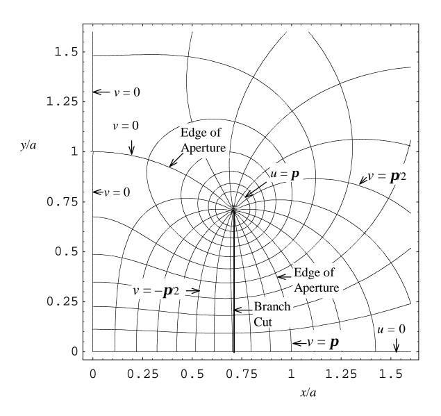
Figure 2.2. Contour map for  $w_4(\mathbf{z})$ . Increments for both u and v are  $\mathbf{p}/10$ .
