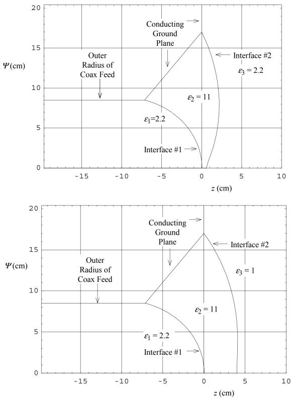
Figure 5.2. Lens design for the oil-lens-oil case (top) and the oil-lens-air case (bottom), with  $\Delta \theta_1 = 50^\circ$ , and  $\Psi_2/\Psi_1 = 2$ .
