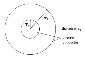
Figure 5.1. A coaxial geometry.
