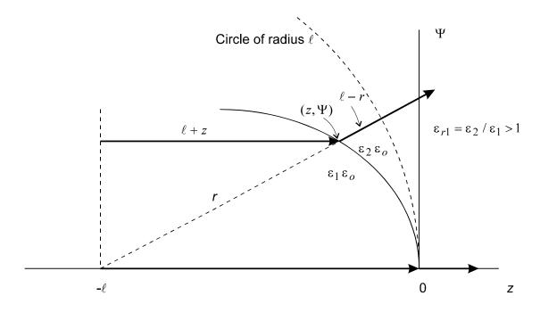
Figure 2.1. Geometry for Interface #1: Prolate spheroidal interface for converting a plane wave to a spherical wave.
