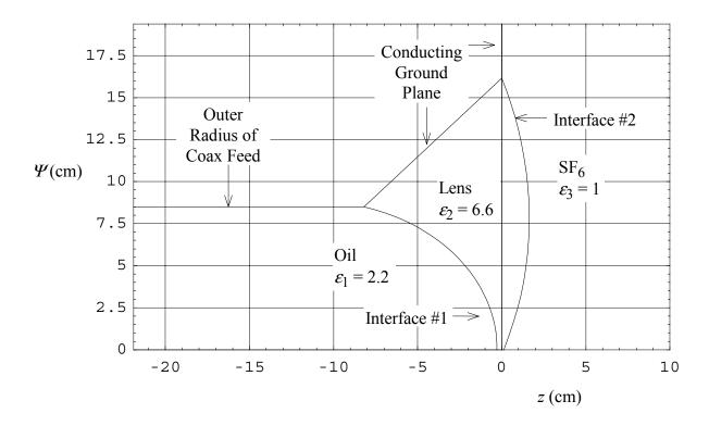
Figure 5.3. Improved oil-lens-air design using  $\Delta \theta_1 = 43^\circ$ , and  $\Psi_2/\Psi_1 = 2$ .
