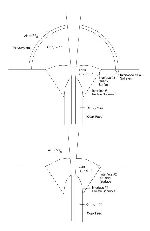
Figure 1.2. Two lens designs, including an oil cap (top) and without an oil cap (bottom).
