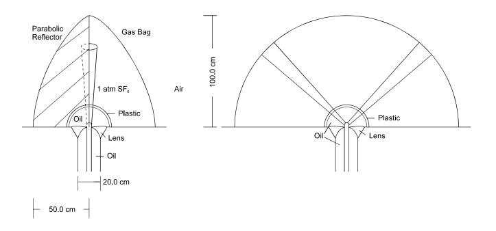
Figure 1.1 A sketch of the Half IRA, shown here with an oil cap.
