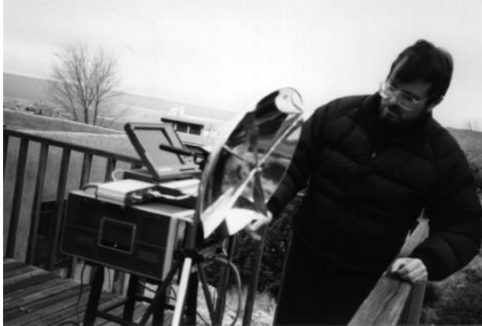
Figure 9.11. The receiving IRA at the outdoor test location.
