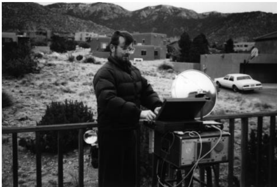
Figure 9.12. The outdoor test site, showing both the receiving IRA (foreground), and the transmitting IRA (behind Dr. Frost).
