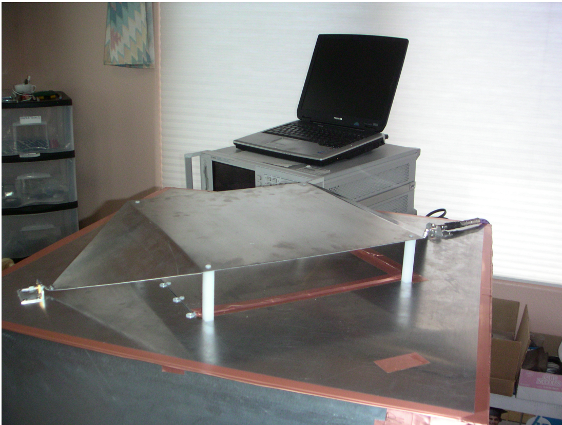
Figure 17. Exterior of the box, showing the stripline (or “blanket”), terminated in 50 \Omega .
