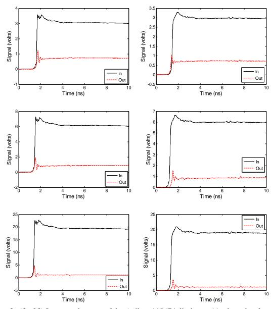
Figure 3. (3 of 3) Inputs and output of the Agilent 11867A limiter at 11voltage levels and 2 polarities, positive polarity on left, negative on right.
