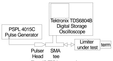
Figure 12. TDR instrumentation.
