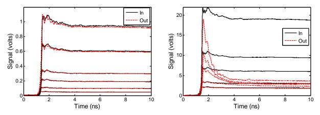
Figure 6. Anitsu 1N50B limiter, positive input.
