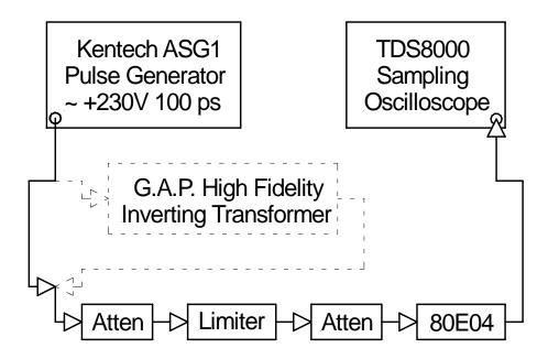
Figure 2. Limiter test setup.
