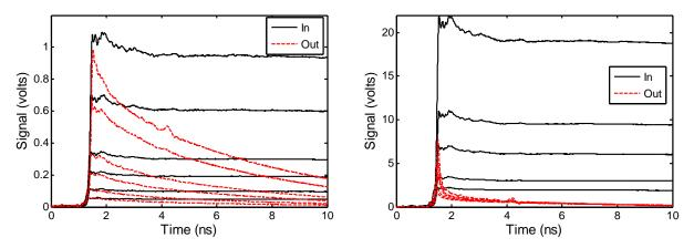
Figure 10. Midisco MDC1527Y-2 1F limiter, positive input.
