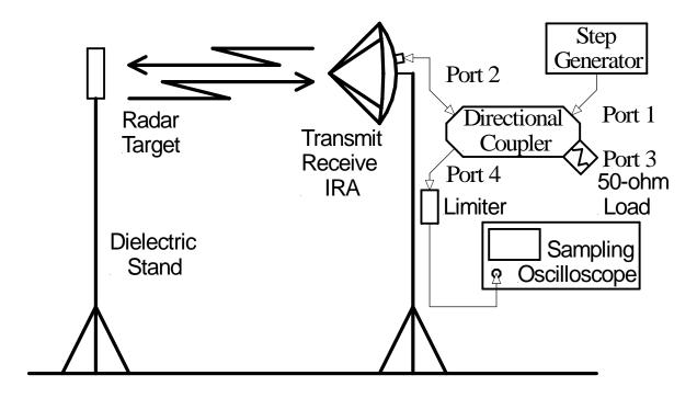
Figure 1. Generic impulse radar instrumentation using a directional coupler.
