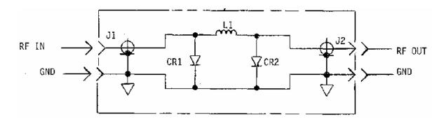
Figure 5. Schematic diagram of the Agilent 11693A limiter.
