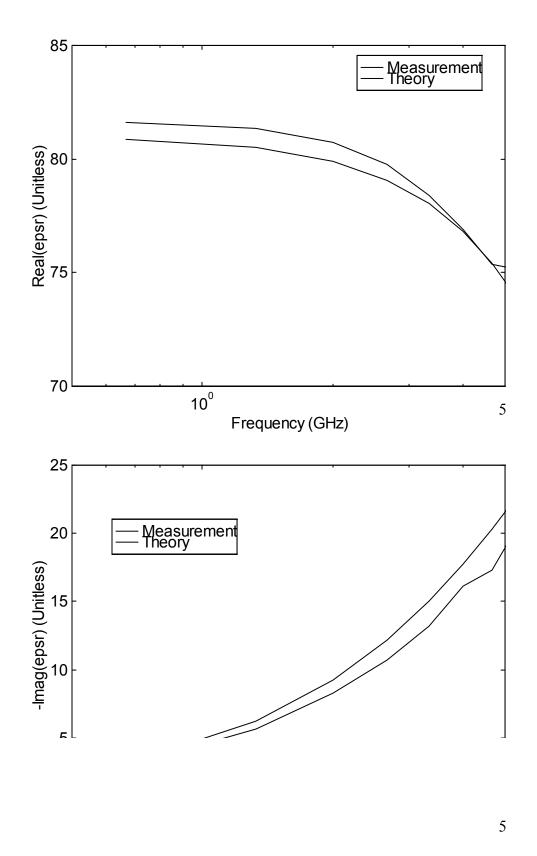
Figure 4.8. Real (top) and imaginary (bottom) parts of the measured dielectric constants of distilled water, measured with water columns 2.39 and 9.55 cm in length..
