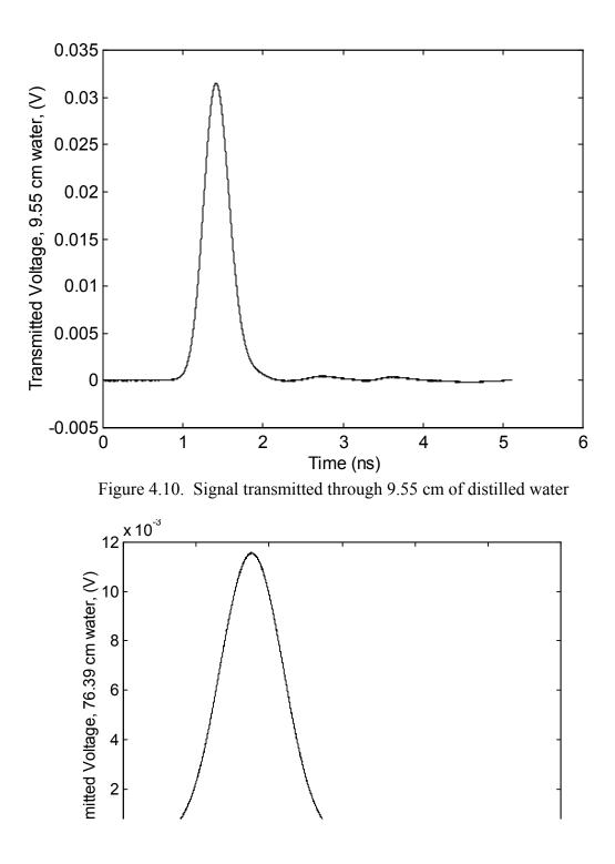
Figure 4.11. Signal transmitted through 76.39 cm of distilled water
