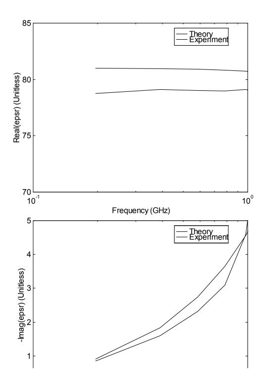
Figure 4.12. Real (top) and imaginary (bottom) parts of the measured dielectric constants of distilled water, using water columns 9.55 and 76.39 cm in length.
