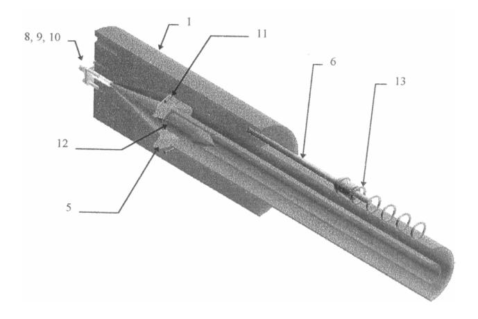
Figure 3.4. Conical expansion section.
