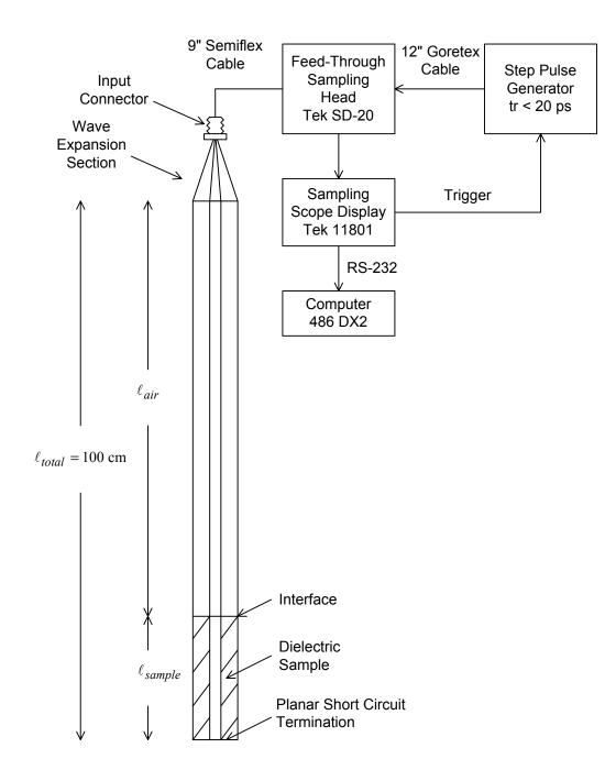
Figure 3.1. Instrumentation setup for measurements in TDR mode.
