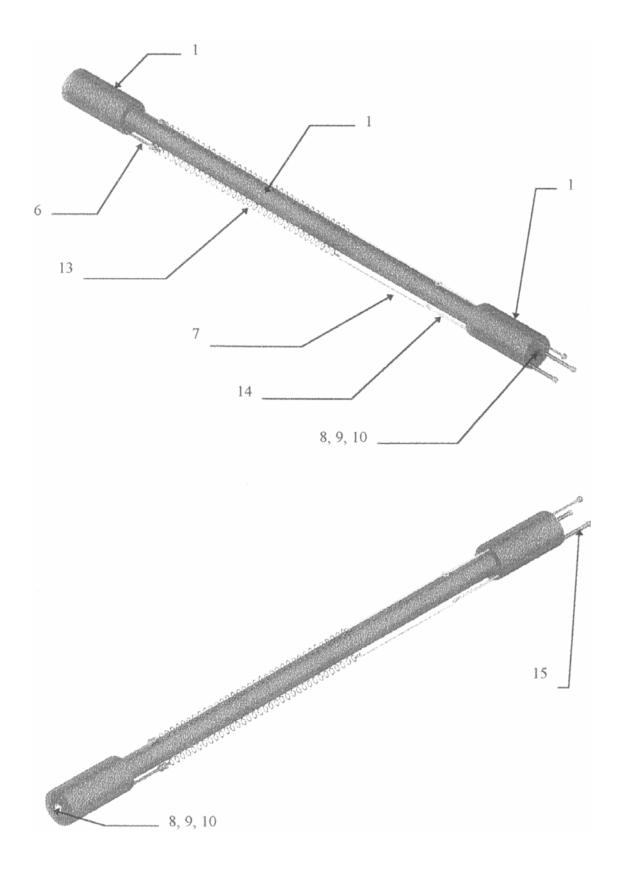
Figure 3.3. Coaxial transmission line apparatus.
