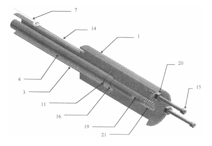
Figure 3.5. Planar short circuit.
